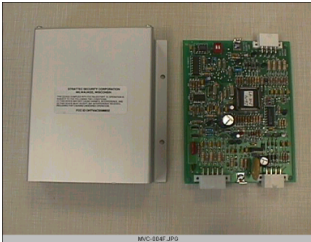
Strattec - Ignition Module PCB open for inspection
