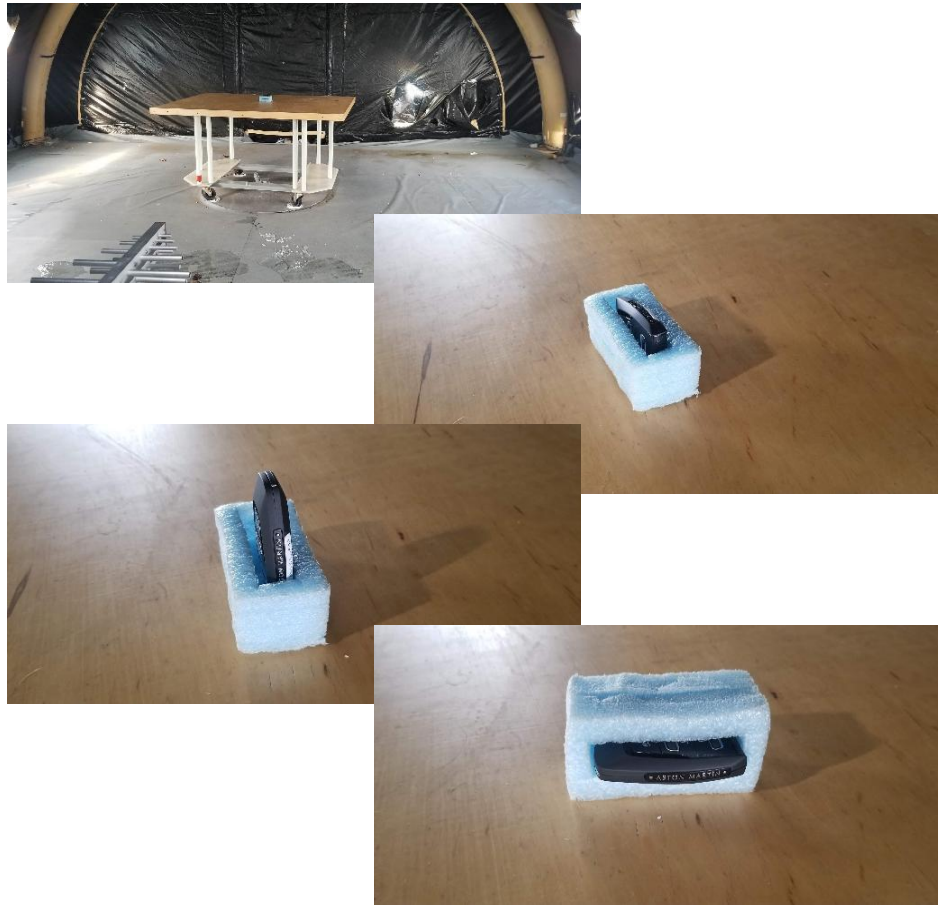
Figure 4: Radiated Emissions Test Setup Photograph(s).
