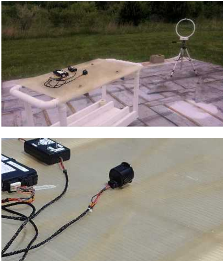
Figure 4: Radiated Emissions Test Setup Photograph(s).
