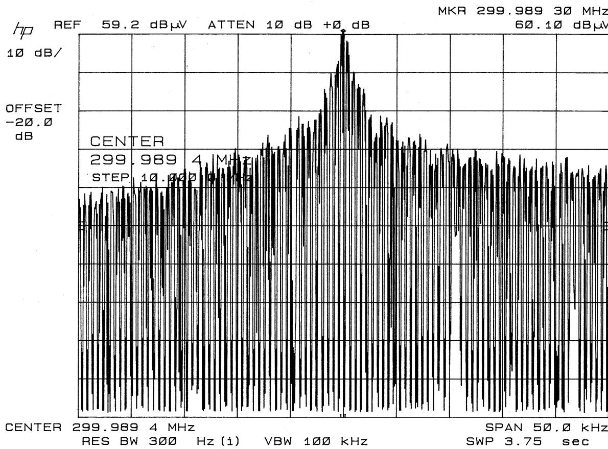
**METHOD OF MEASUREMENT:** A small sample of the transmitter output was fed into the spectrum analyzer and the above plot was generated. The vertical scale is set to 10 dB per division: the horizontal scale is set to 5 kHz per division.
