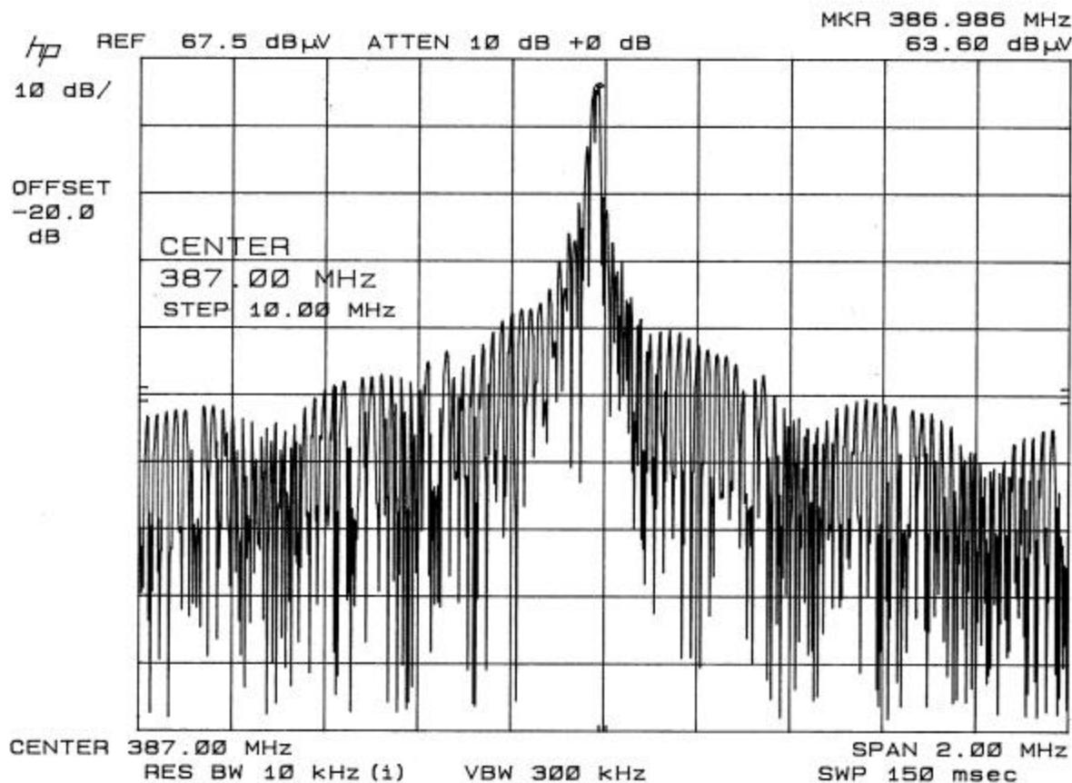
**METHOD OF MEASUREMENT:** A small sample of the transmitter output was fed into the spectrum analyzer and the above plot was generated. The vertical scale is set to 10 dB per division: the horizontal scale is set to 200 kHz per division.
