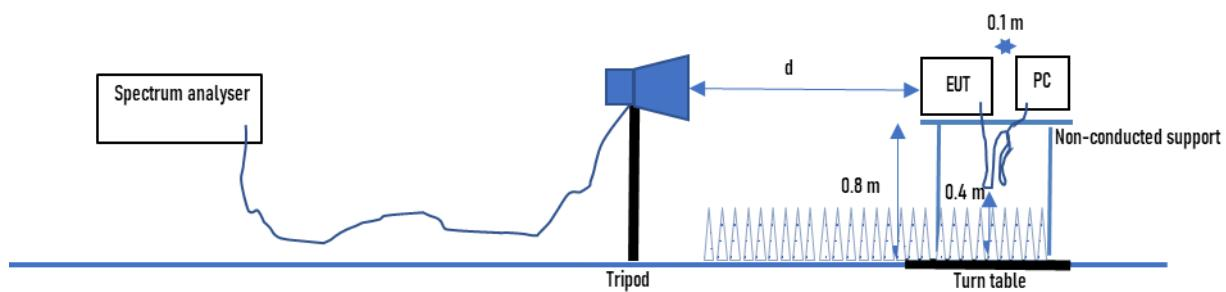
Radiated emission from the EUT are measured in the frequency range of 1 GHz to the maximum frequency as specified in 47 CFR Part 15 Subpart A section 15.33, using a tuned receiver (spectrum analyser) and appropriate linearly polarized antennas. Table top equipment is placed on a 0.65 X 1.0 metre non-conducting table 80 centimetres above the ground plane. The turntable is fully covered with the appropriate absorber (Type VHP-12).
