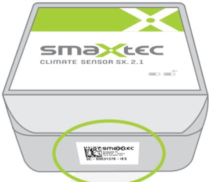
First, add the Climate Sensor to your organisation in the smaXtec Messenger via "Boluses & Devices". Use the serial number printed on the side label and add a name in the „Add device“ screen. The location of the device is suitable as a name, e.g. „calving area“, „dry cow barn“ or „fresh cows“.
