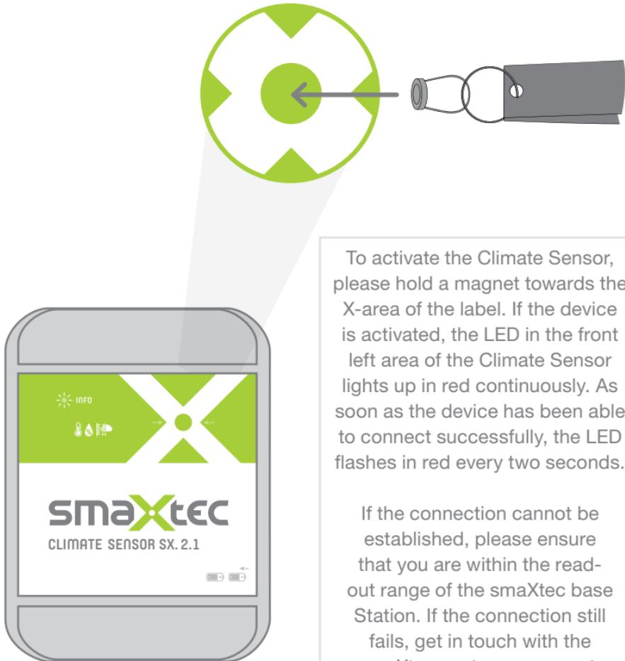
To activate the Climate Sensor, please hold a magnet towards the X-area of the label. If the device is activated, the LED in the front left area of the Climate Sensor lights up in red continuously. As soon as the device has been able to connect successfully, the LED flashes in red every two seconds.
