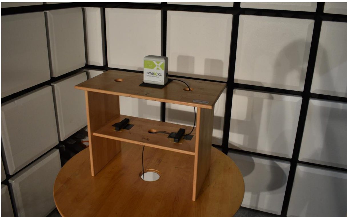
Figure 1-2: Measurement setup principal picture of DUT, Position 0°
