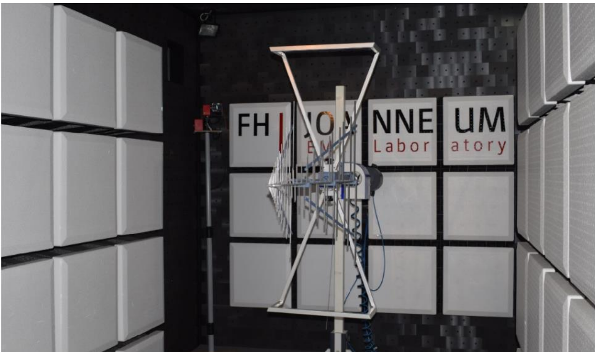
Figure 4: Ultra Log antenna in vertical polarization.
