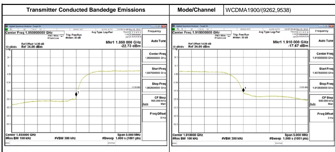
Note: "ALIGN OFF" means that we turn off the auto align. We align the spectrum at each time before test.
