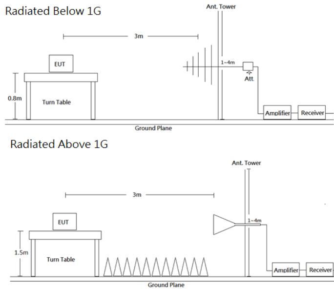
Radiated emission tests were performed in the 3 meters chamber test site, using the setup accordance with the ANSI C63.10-2013. The specification used was the FCC Part 15.209 and FCC 15.247 Limits.
