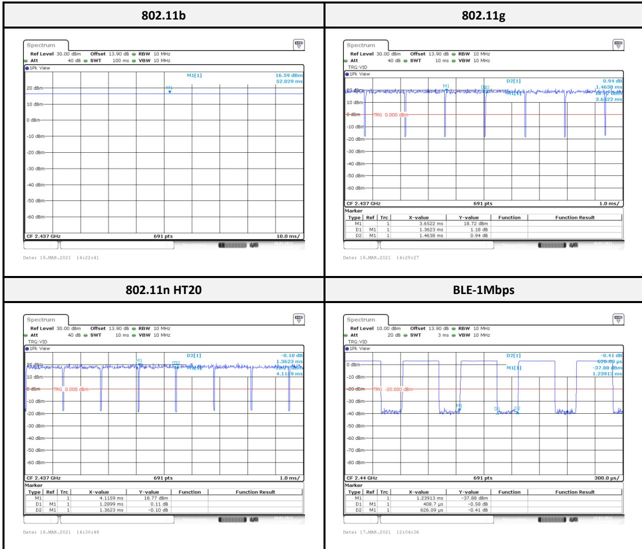
\*Note: Duty Factor =  $10 \times \log(1/\text{Duty cycle})$
