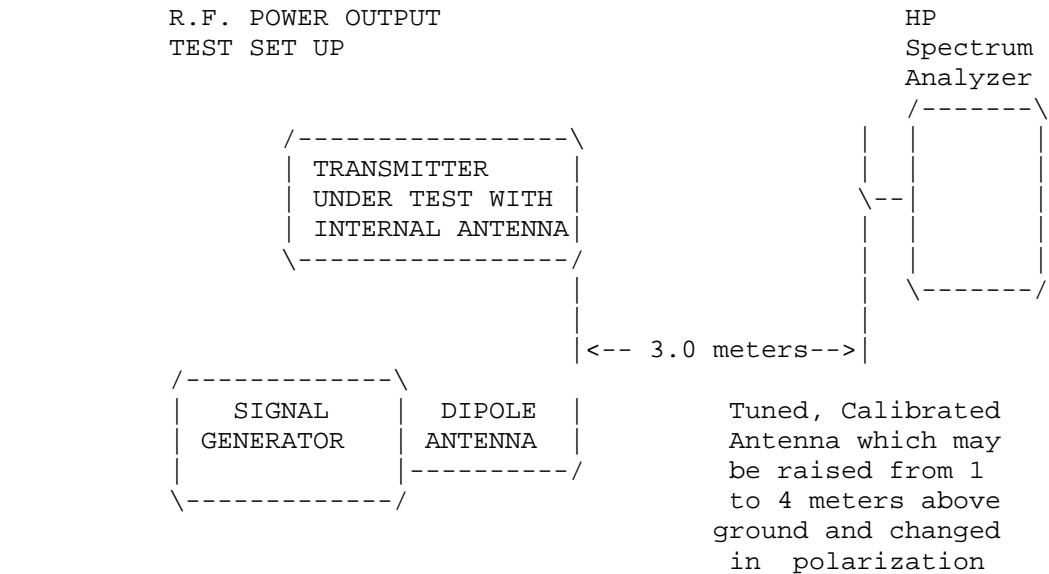
Equipment placed 1 meter above ground
