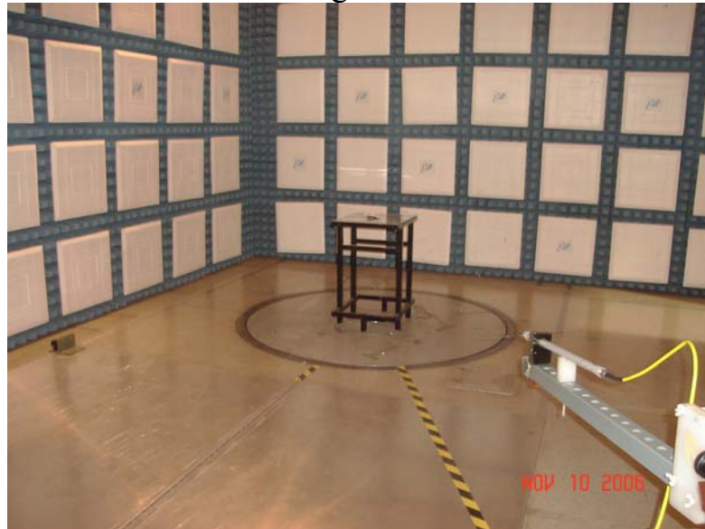
Test Set-up for Radiated Emissions Horizontal Polarity
