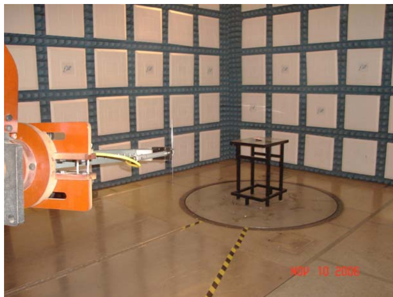
Test Set-up for Radiated Emissions Vertical Polarity
