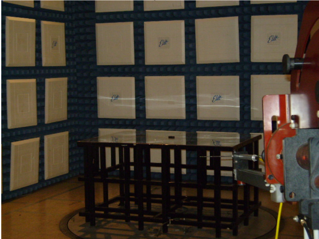
Test Set-up for Radiated Emissions – Horizontal Polarity
