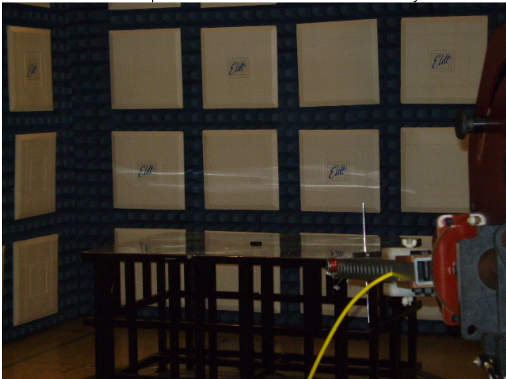
Test Set-up for Radiated Emissions – Vertical Polarity
