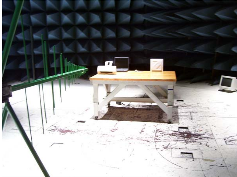
Photograph 4. Radiated Emission Test Setup 30 MHz - 1 GHz, Front View
