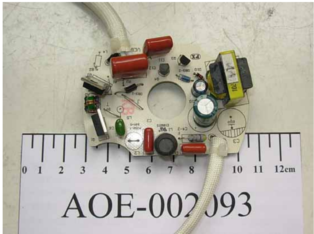
FIGURE 2 BALLAST (M/N: VEB82122) MAIN BOARD (COMPONENT SIDE)
