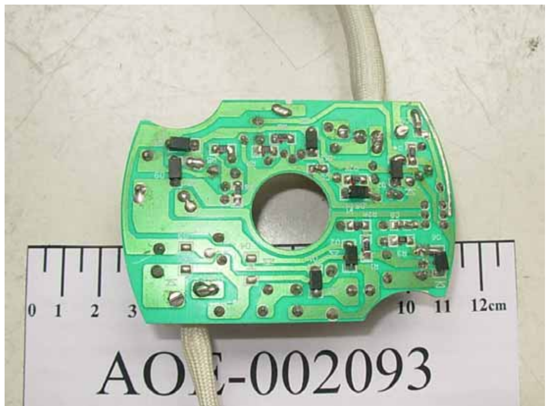
FIGURE 12 BALLAST (M/N: VEB82140) MAIN BOARD (SOLDERED SIDE)
