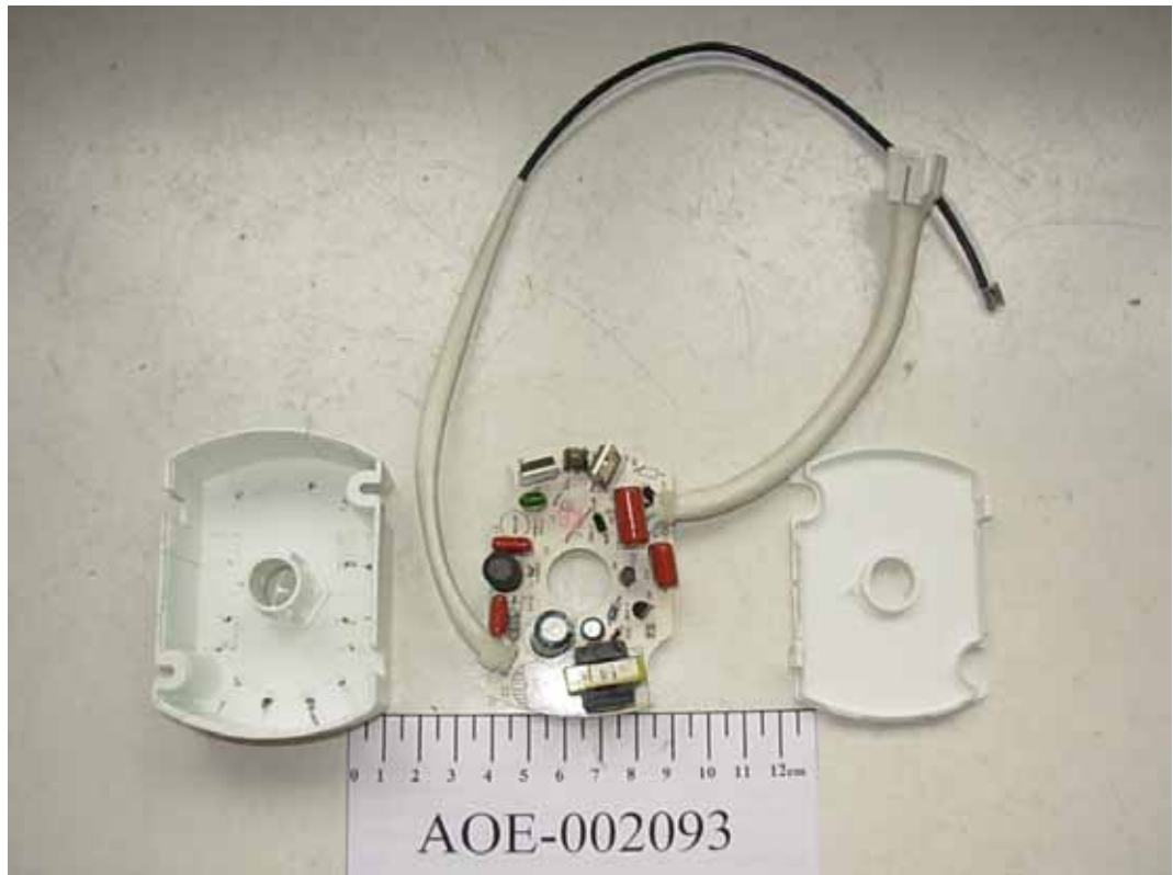
FIGURE 1 BALLAST (M/N: VEB82122) COVER REMOVED
