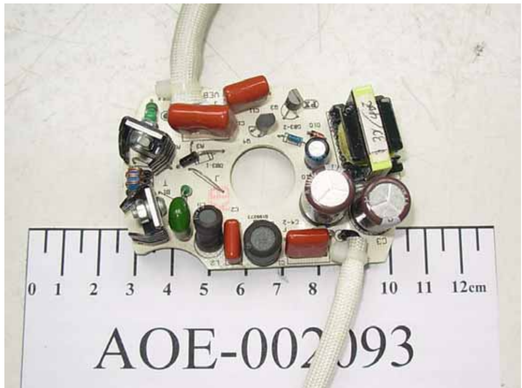
FIGURE 11 BALLAST (M/N: VEB82140) MAIN BOARD (COMPONENT SIDE)
