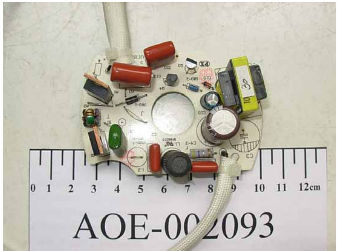
FIGURE 5 BALLAST (M/N: VEB82130) MAIN BOARD (COMPONENT SIDE)
