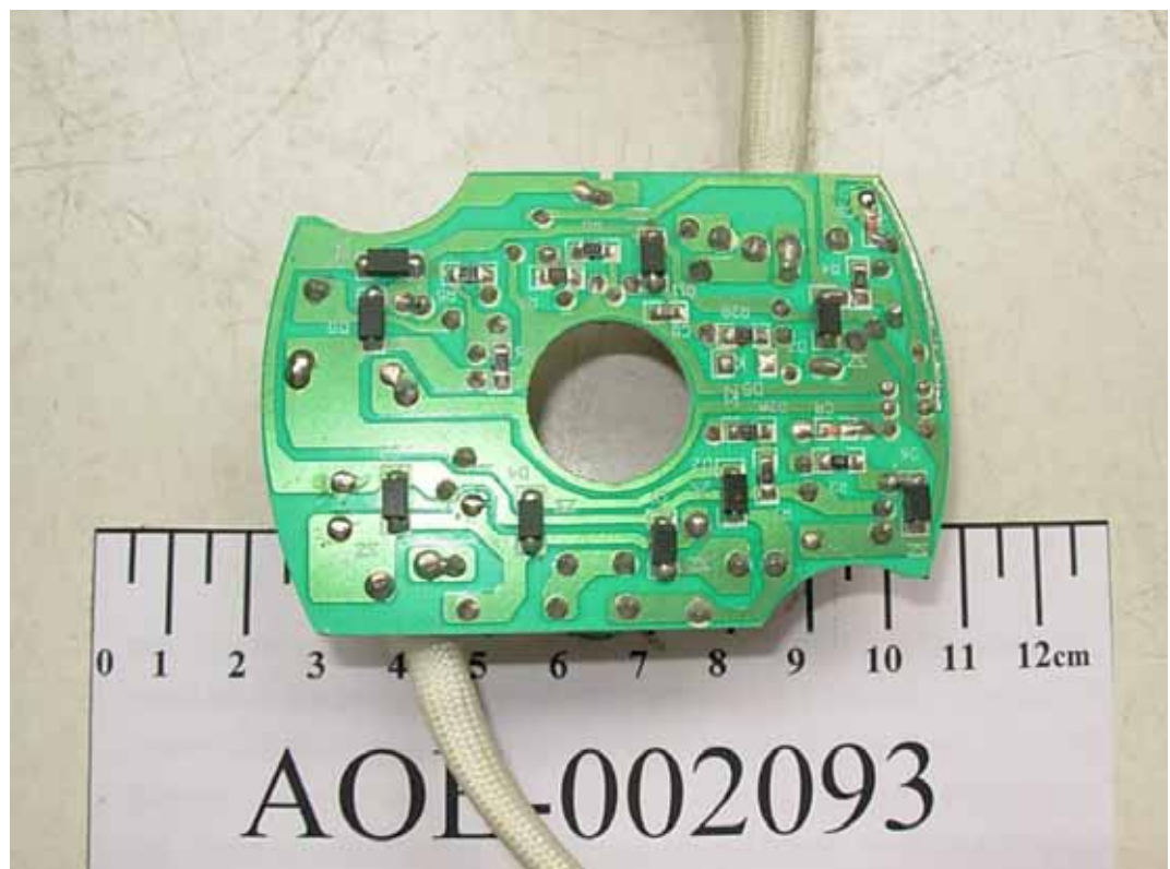
FIGURE 6 BALLAST (M/N: VEB82130) MAIN BOARD (SOLDERED SIDE)
