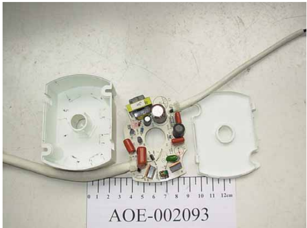
FIGURE 4 BALLAST (M/N: VEB82130) COVER REMOVED
