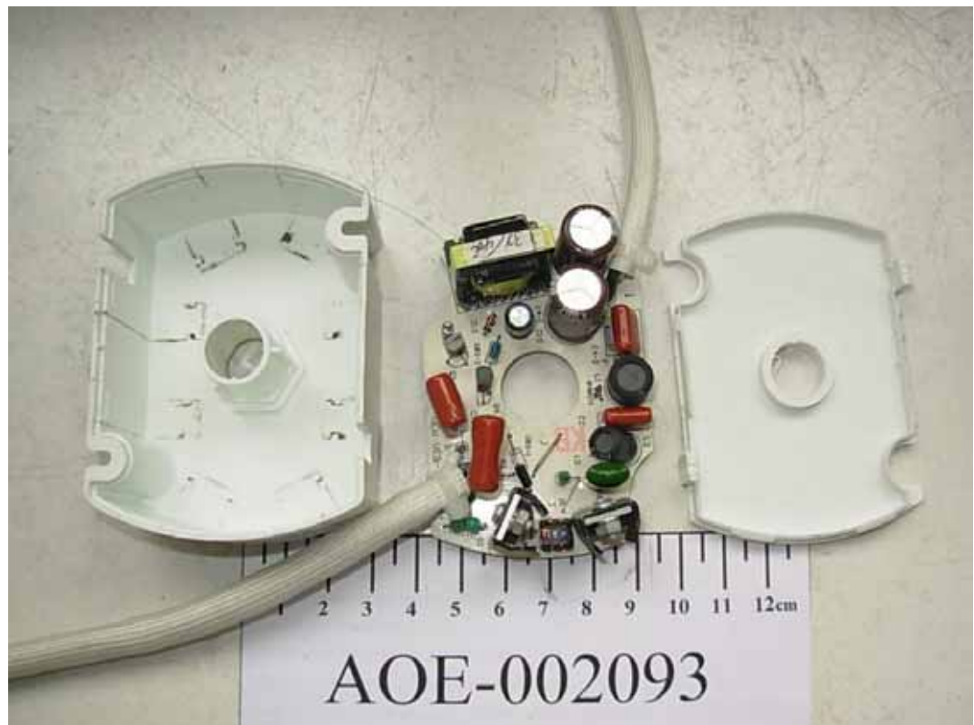
FIGURE 7 BALLAST (M/N: VEB82132) COVER REMOVED
