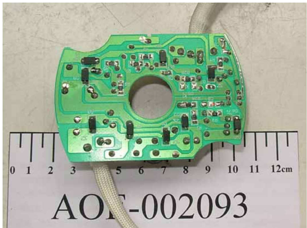
FIGURE 3 BALLAST (M/N: VEB82122) MAIN BOARD (SOLDERED SIDE)
