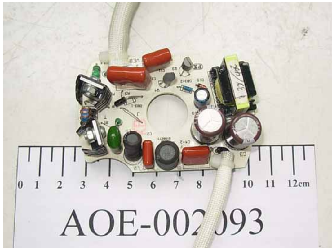
FIGURE 8 BALLAST (M/N: VEB82132) MAIN BOARD (COMPONENT SIDE)
