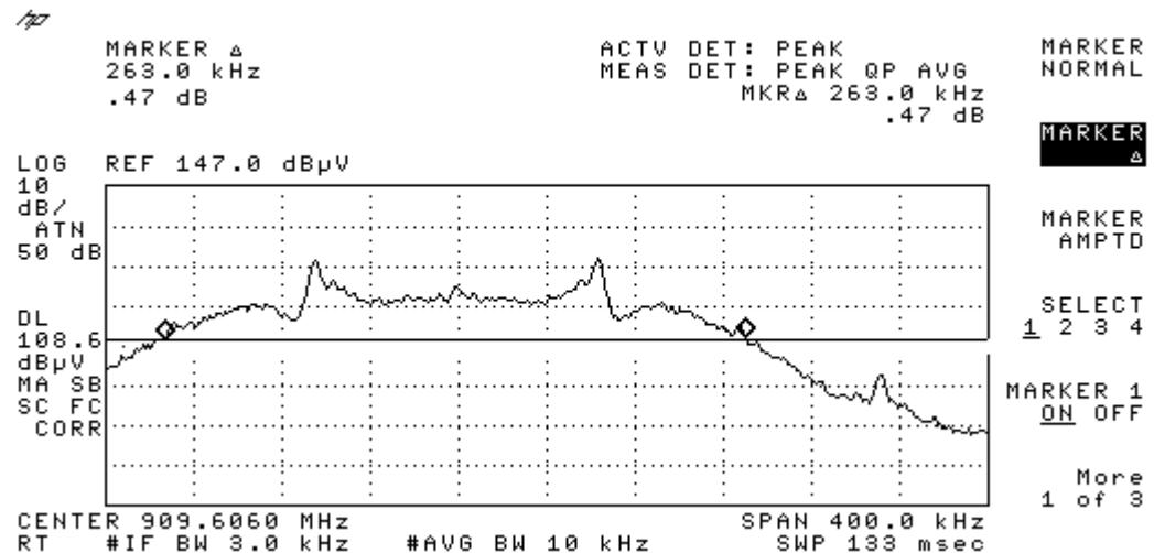
Conducted 20 dB BW Measurement at Antenna Port(s) 47 CFR 15.247(a)(1)
