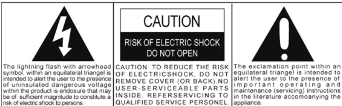
The Caution Marking is located at the bottom of the apparatus.
