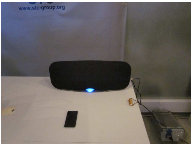
Measurement of Conducted Emission Test Set Up
