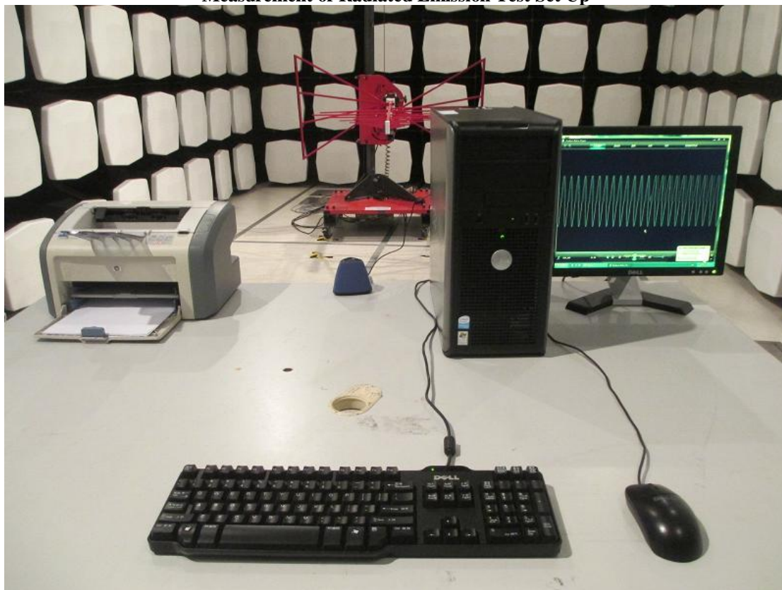
Measurement of Radiated Emission Test Set Up
