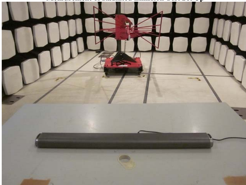
Measurement of Radiated Emission Test Set Up
