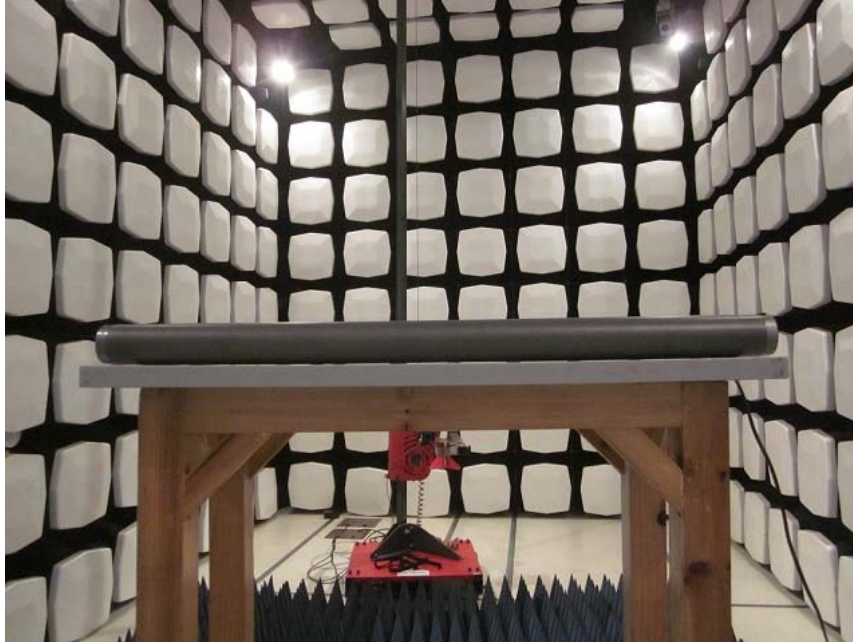
Measurement of Radiated Emission Test Set Up
