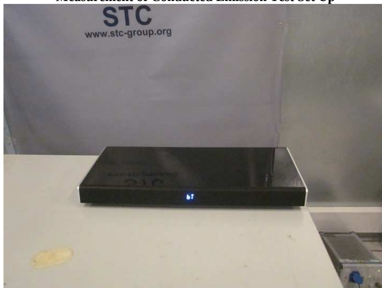
Measurement of Conducted Emission Test Set Up
