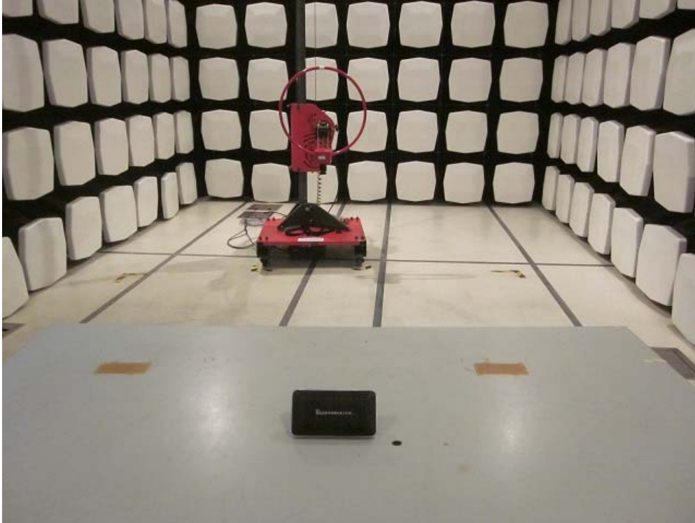
Measurement of Radiated Emission Test Set Up
