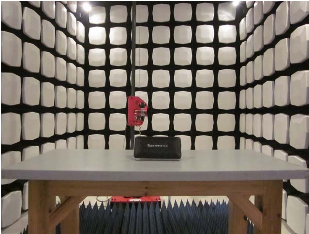
Measurement of Radiated Emission Test Set Up
