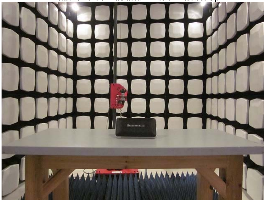
Measurement of Radiated Emission Test Set Up
