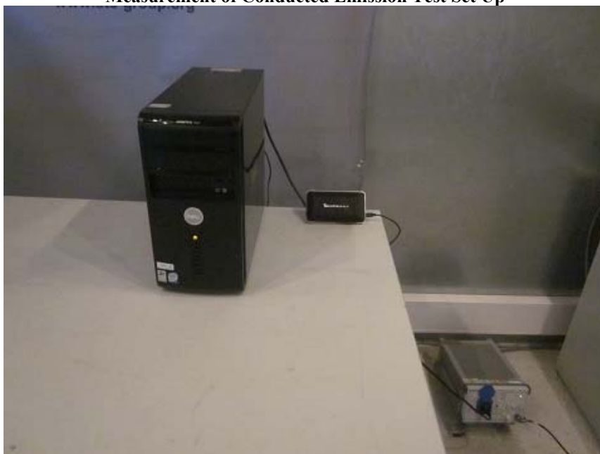
Measurement of Conducted Emission Test Set Up
