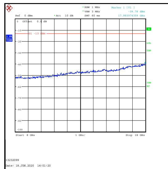
**Transmitter Out of Band Radiated Emissions (Bluetooth LE & UMTS Band V) (continued)**
