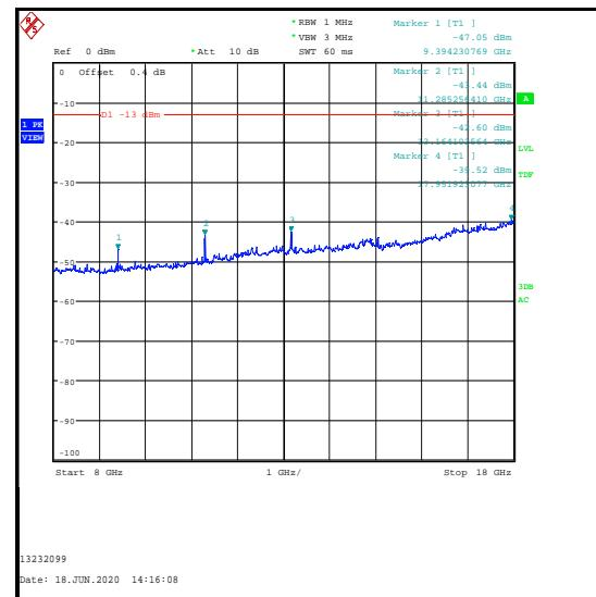
**Transmitter Out of Band Radiated Emissions (Bluetooth LE & UMTS Band II) (continued)**
