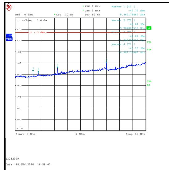
**Transmitter Out of Band Radiated Emissions (Bluetooth LE & LTE Band 2) (continued)**
