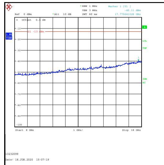
**Transmitter Out of Band Radiated Emissions (Bluetooth LE & LTE Band 13) (continued)**
