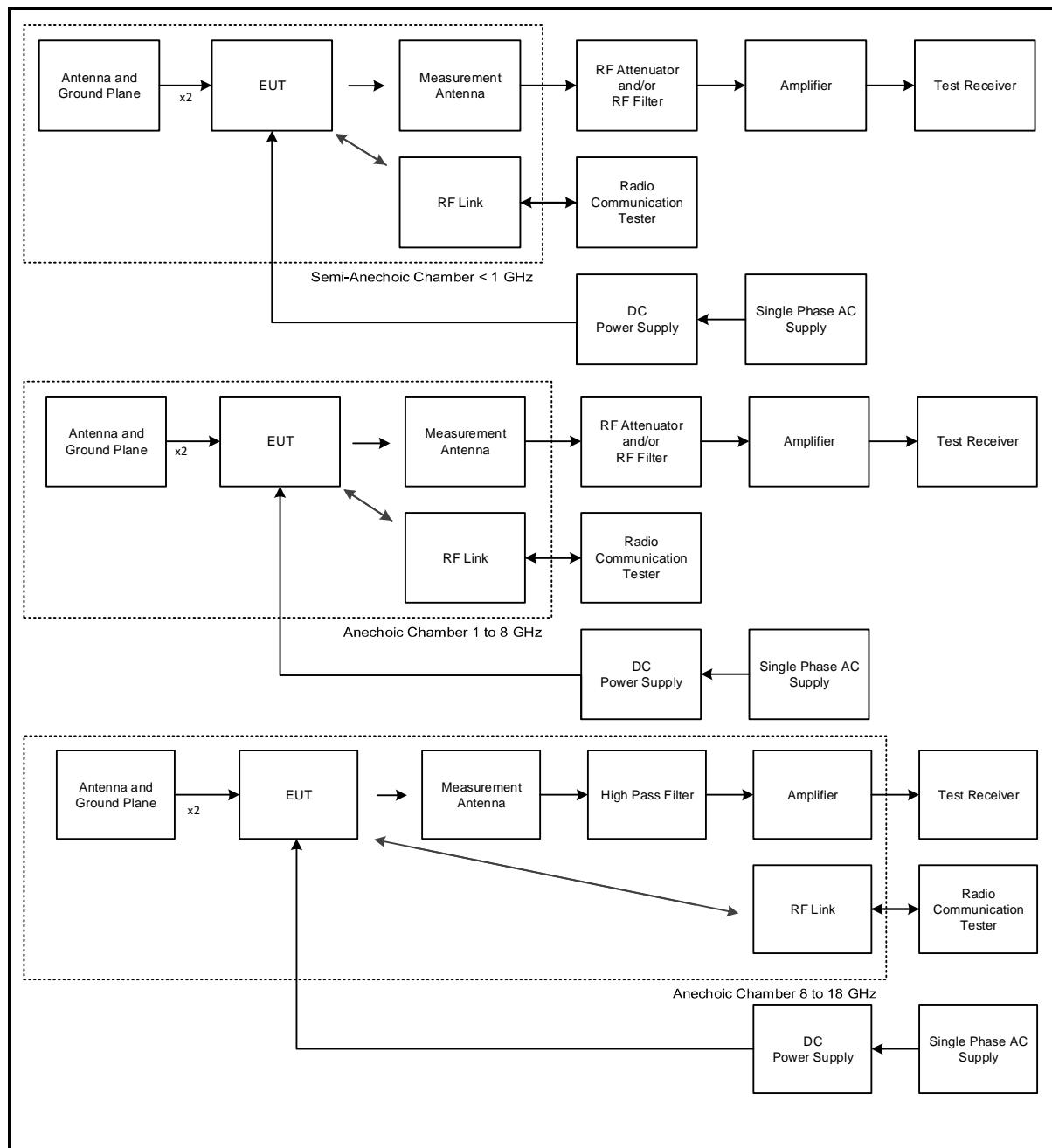
**Test Setup Diagrams (continued)****Transmitter Radiated Emissions**
