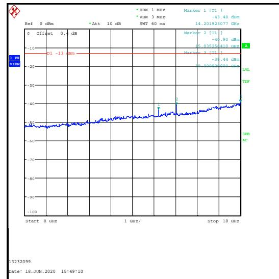
**Transmitter Out of Band Radiated Emissions (Bluetooth LE & LTE Band 5) (continued)**
