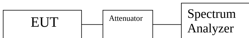
Figure 2. Occupied Bandwidth, Test Setup
