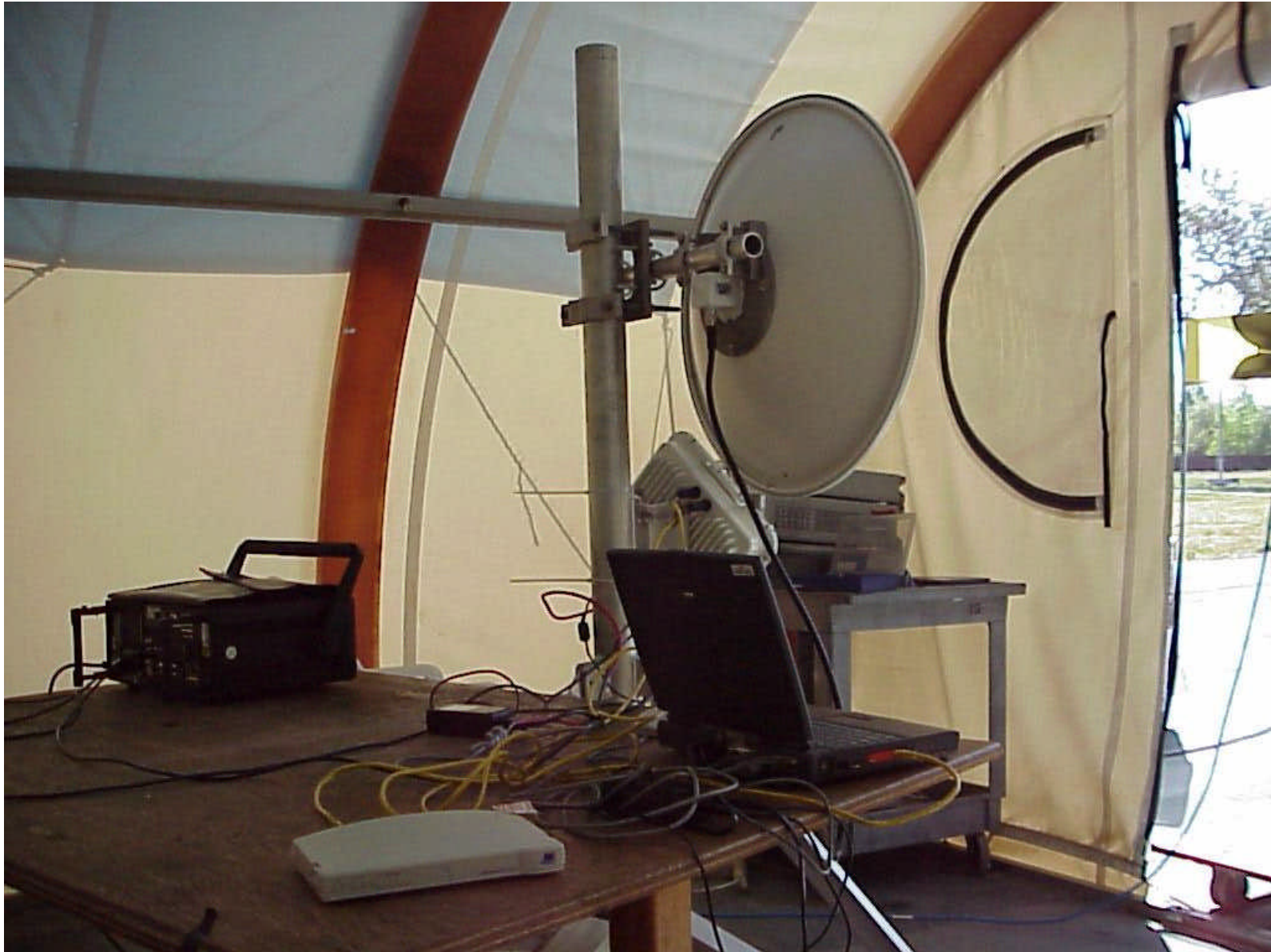
Link CX, 15.205 Radiated emissions, Restricted bands, setup
