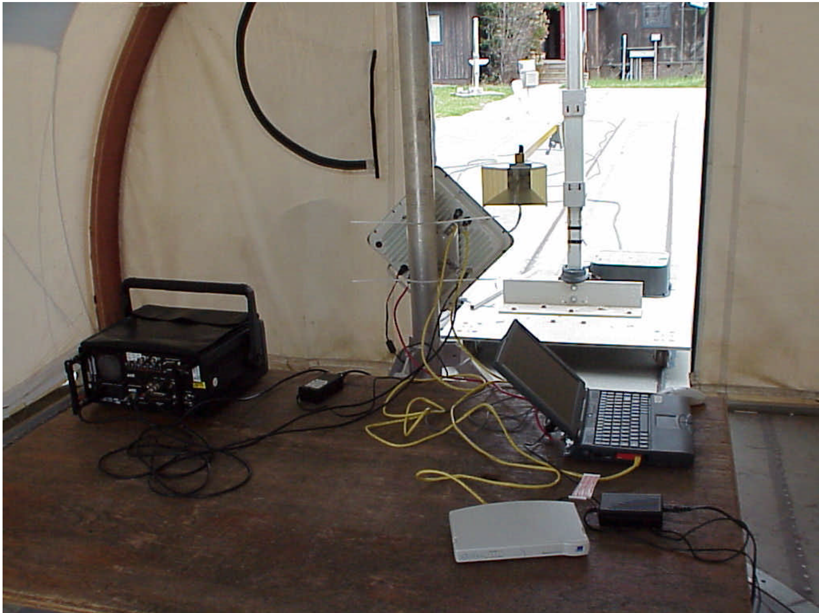
Link CX, 15.205 Radiated emissions, Restricted bands, setup
