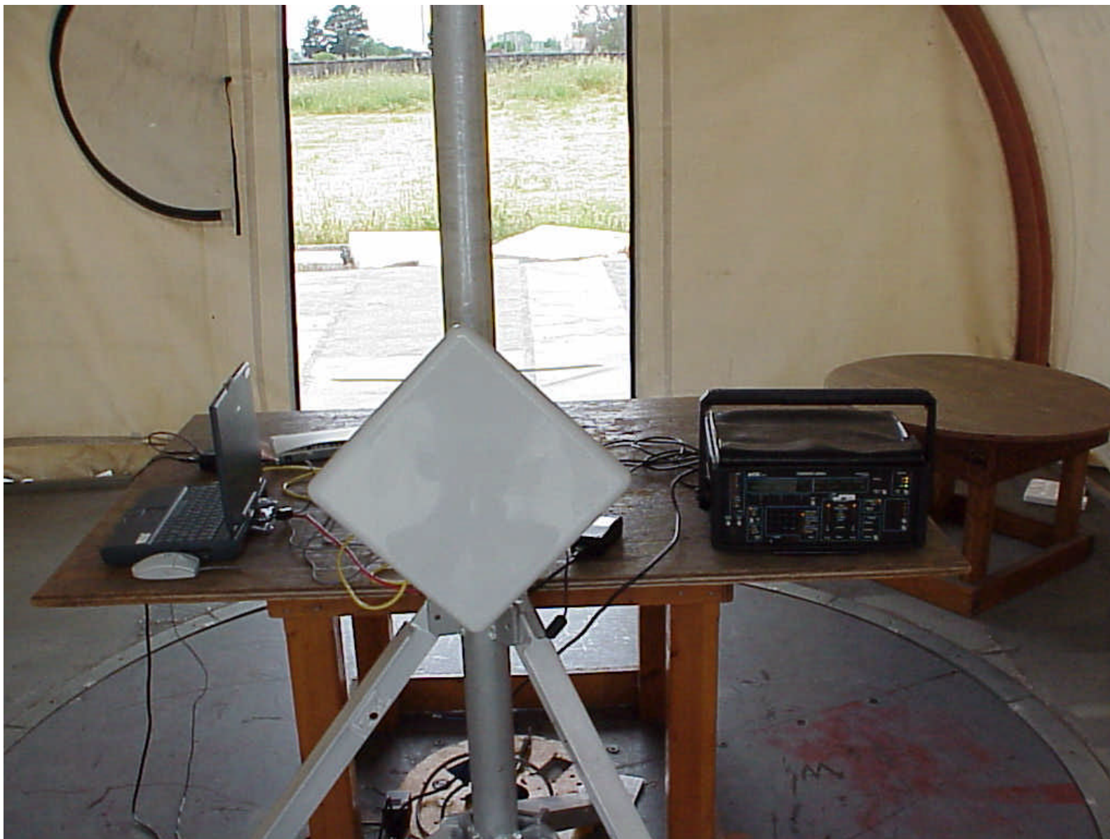
Link CX, 15.205 Radiated emissions, Restricted bands, setup
