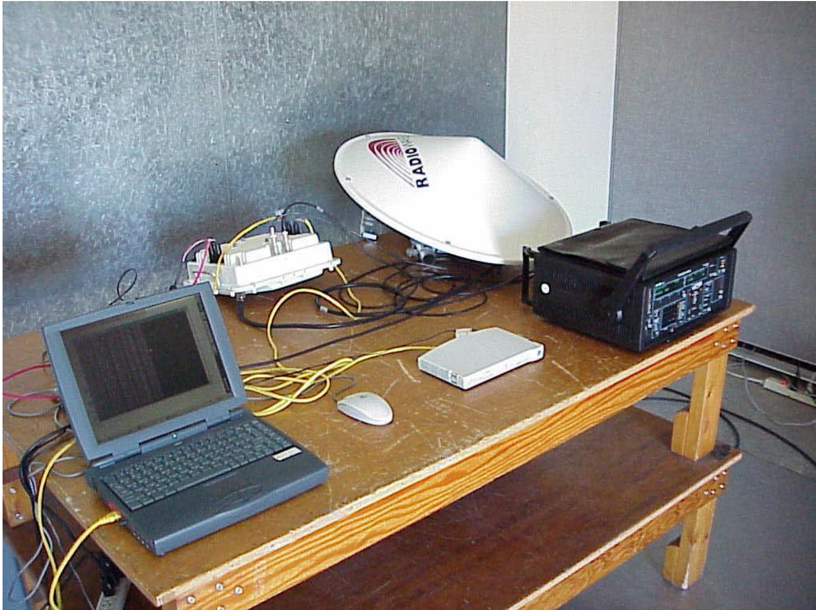
Link CX, AC Line conducted emissions setup photo
