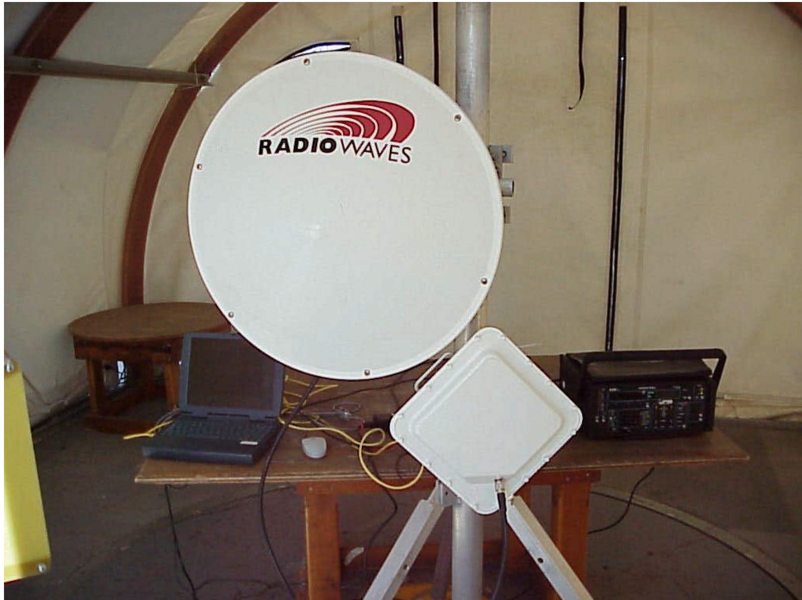
Link CX, 15.205 Radiated emissions, Restricted bands, setup
