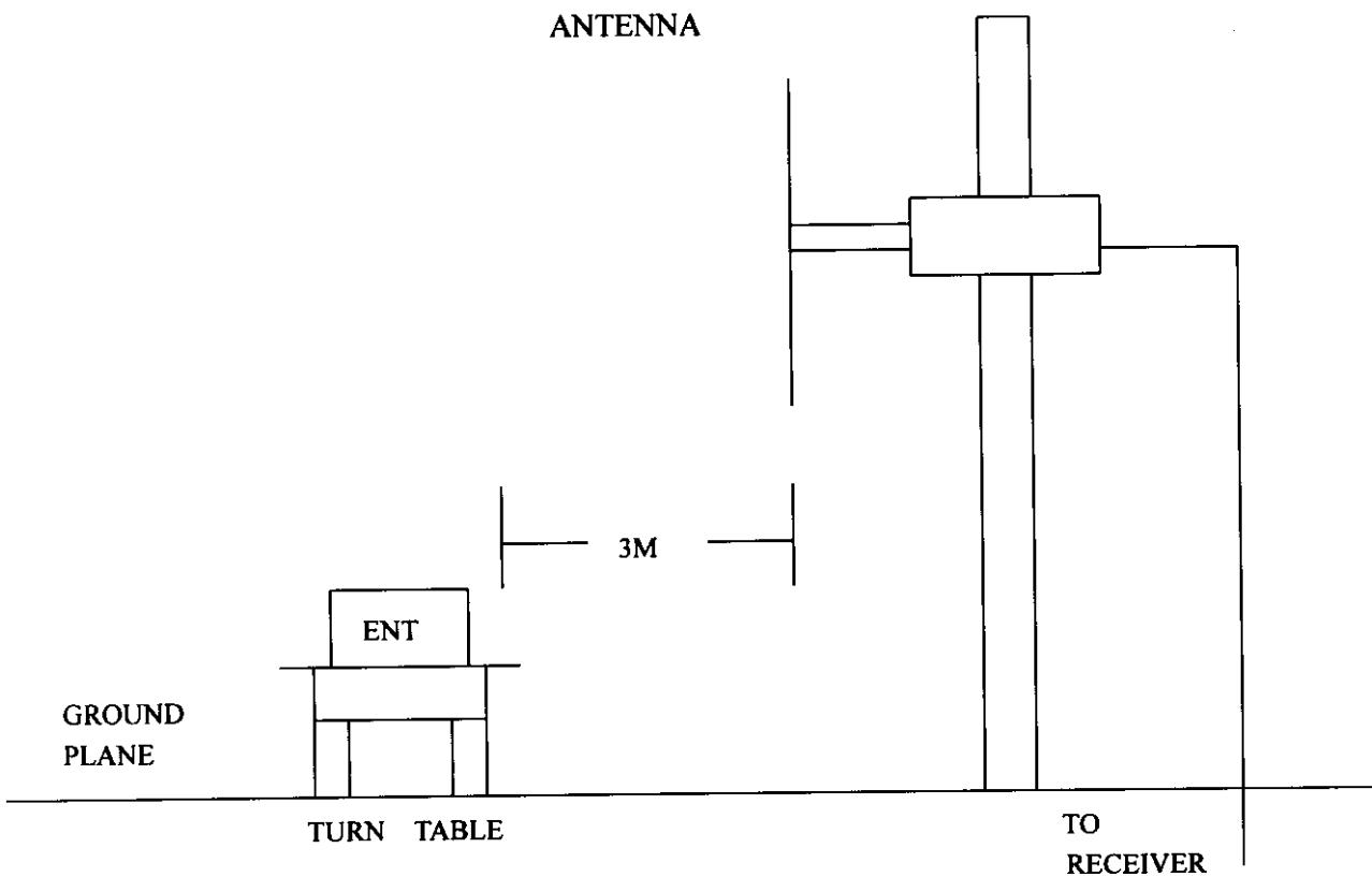
**5 . 3 RADIATED TEST SET-UP**
