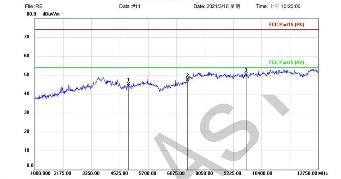
Site: Limit: FCC Part15 (PK) EUT: AOA/AOD M/N: TLSR8278IP48D Mode: TX-2441 Note: Polarization: **Vertical** Power: Distance: 3m Temperature: Humidity: %
