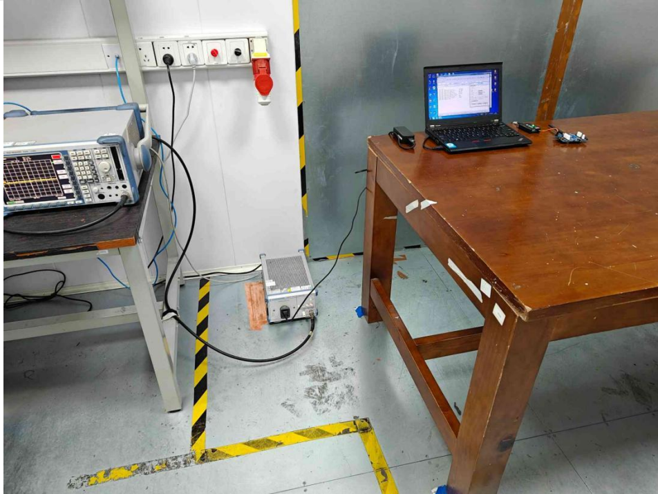
Conducted emissions at AC power line (150kHz-30MHz)
