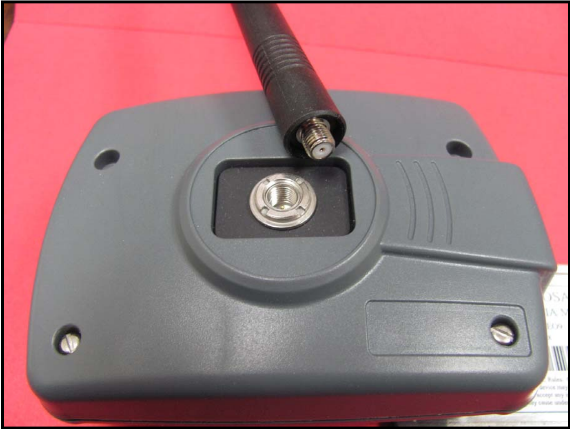
ODYDORE09: External photo, using endcap antenna, reverse SMA closeup.
