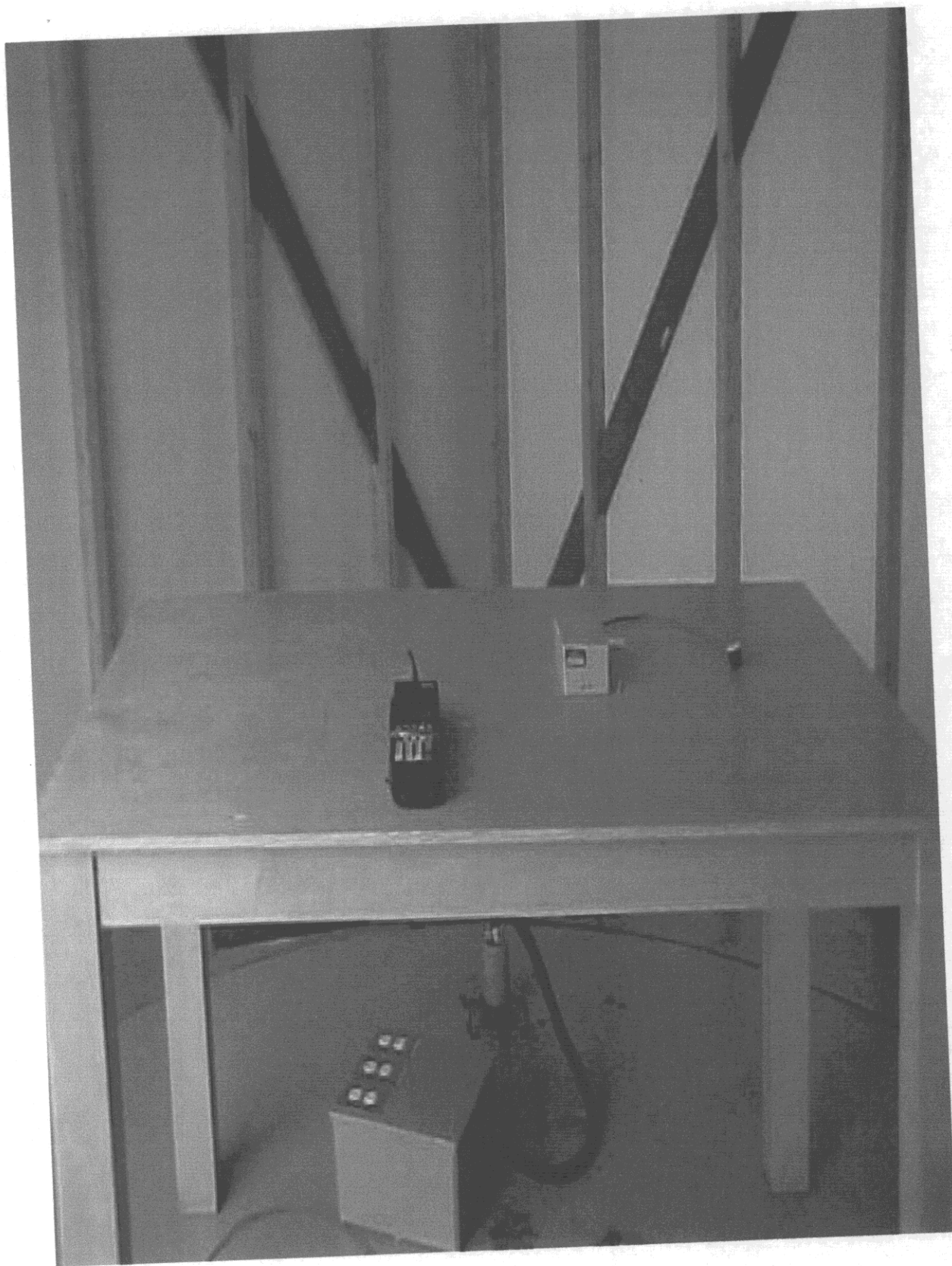
Figure 8 - Radiated Setup (Digital Device/Receiver)
