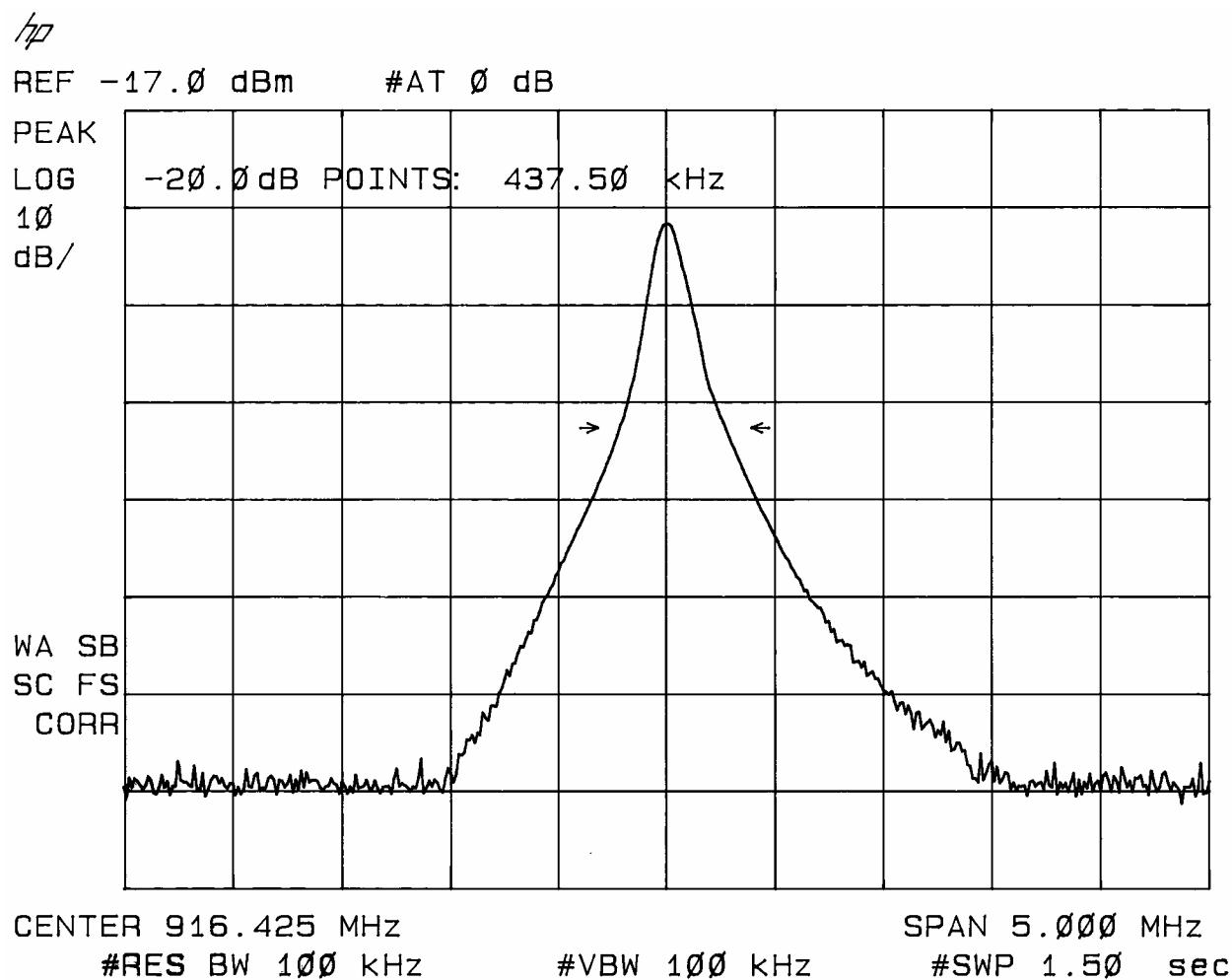
The field strength measurements were taken using an HP8596E spectrum analyzer, an EMCO 3121C dipole set, an EMCO 3115 double ridge guide horn and an Avantek UJ210 preamp. The device was scanned from 30 MHz. to 10 GHz. and all emissions were noted. In this case, the only emissions detected were those harmonically related to the fundamental transmit frequency.
