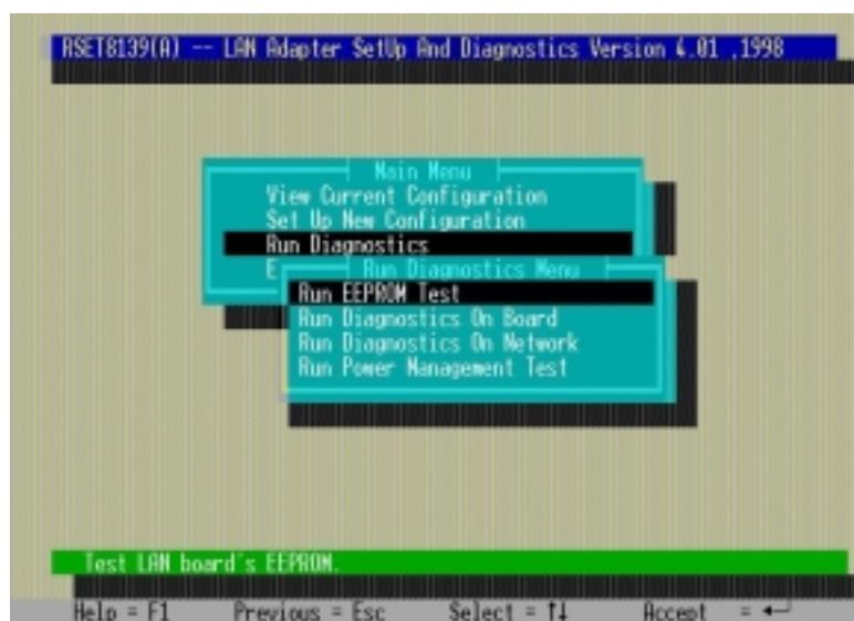
The **Run Diagnostics tests** do a basic function verification on board of LFE-8139TX NIC.
