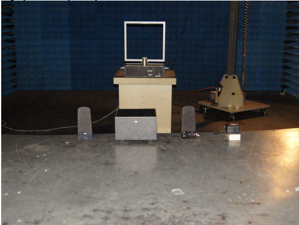
Photograph 2: Set-up for Spurious Emissions for 30 - 1000MHz
