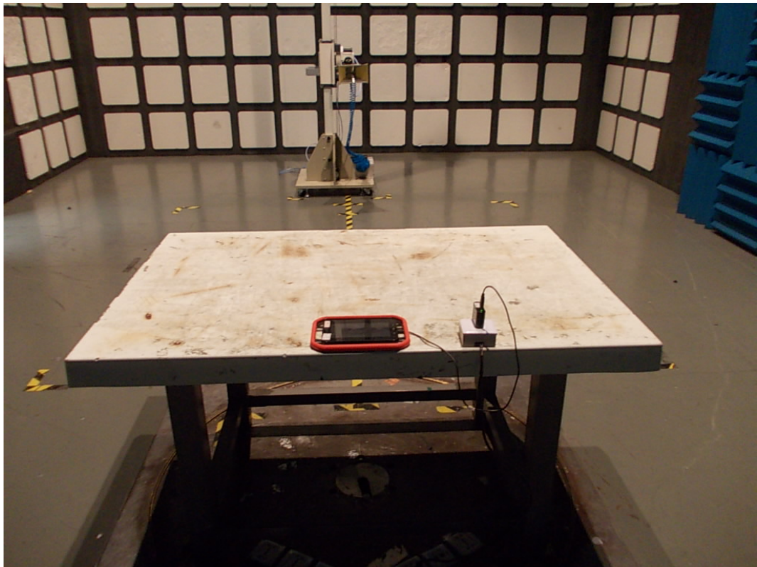
BACK VIEW OF RADIATED EMISSION TEST (ABOVE 1GHz) (TEST MODE: OPERATING (CHARGING WITH ADAPTER))
