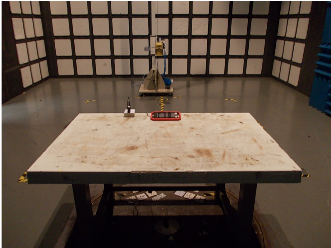
FRONT VIEW OF RADIATED EMISSION TEST (ABOVE 1GHz) (TEST MODE: OPERATING (CHARGING WITH ADAPTER))
