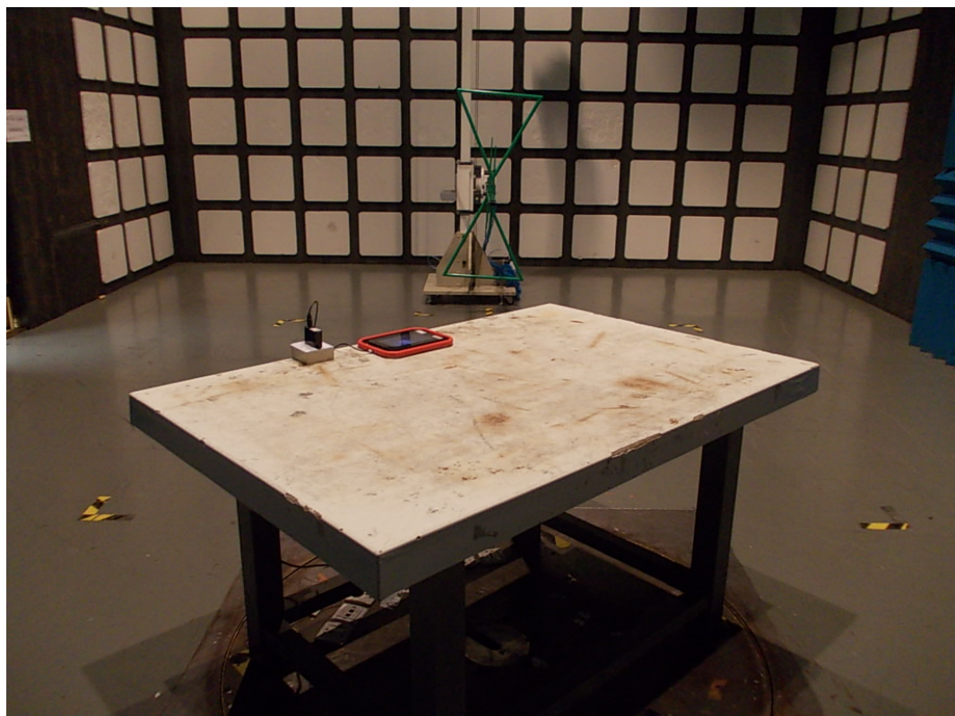
SETUP WITH MAXIMUM DETECTED EMISSION AT VERTICAL POLARIZATION (TEST MODE: OPERATING (CHARGING WITH ADAPTER))
