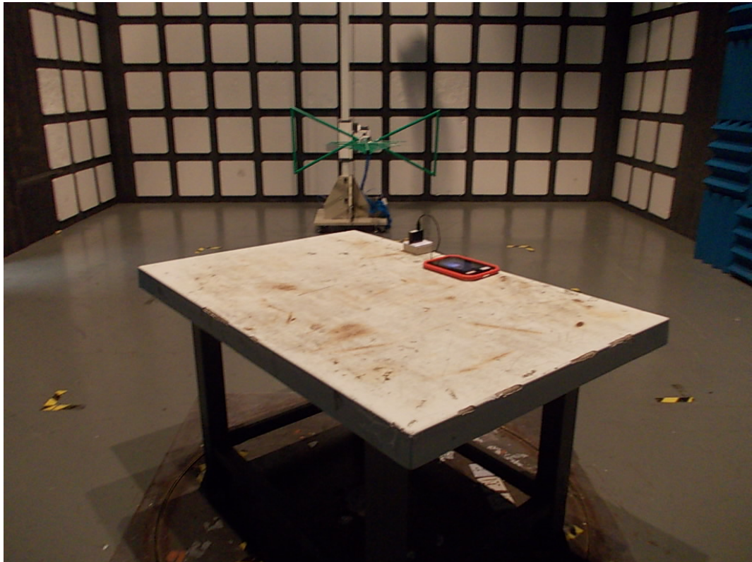
SETUP WITH MAXIMUM DETECTED EMISSION AT HORIZONTAL POLARIZATION (TEST MODE: OPERATING (CHARGING WITH ADAPTER))
