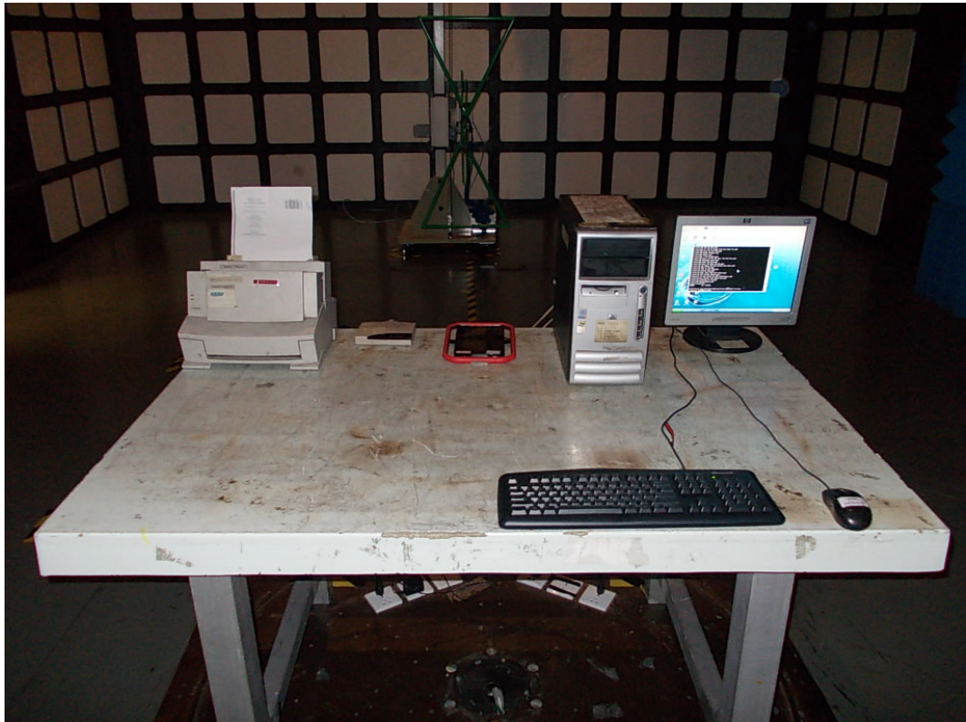
FRONT VIEW OF RADIATED EMISSION TEST (BELOW 1GHZ) (TEST MODE: OPERATING (LINK PC))
