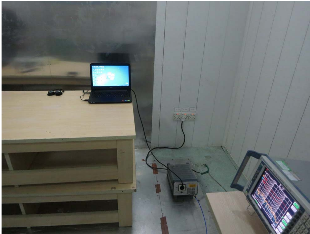
FCC RADIATED EMISSION TEST SETUP
