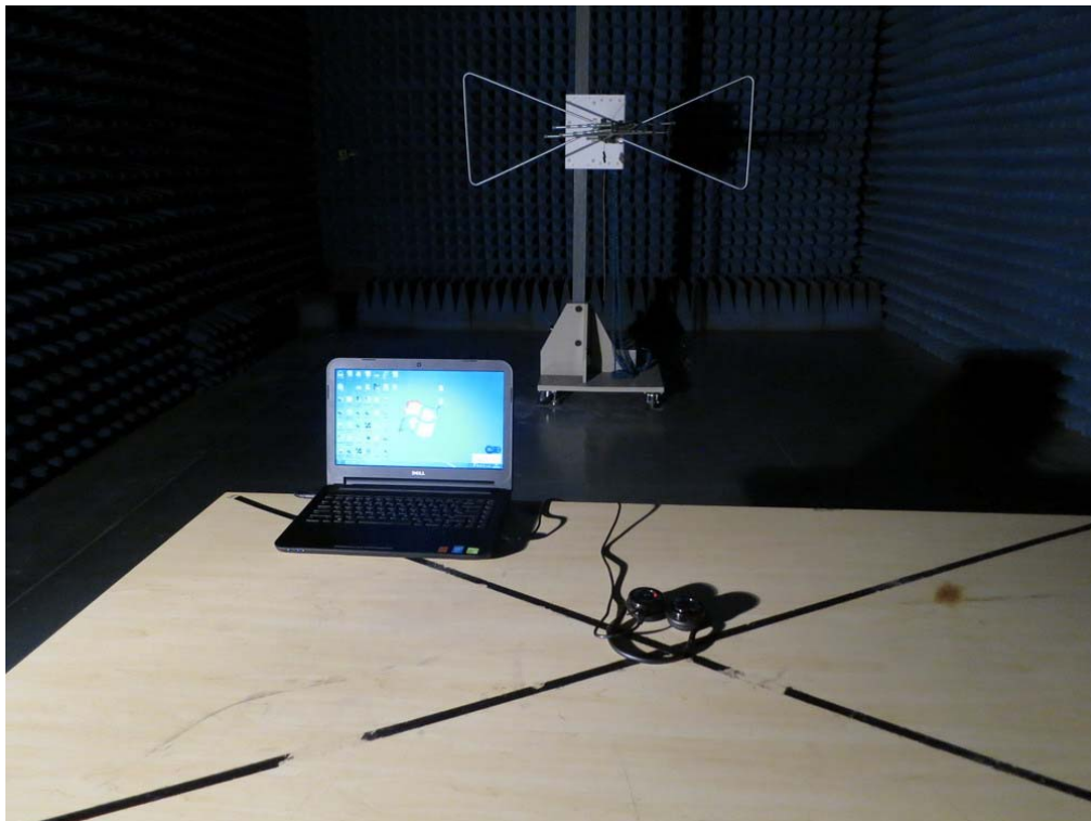
FCC RADIATED EMISSION TEST SETUP
