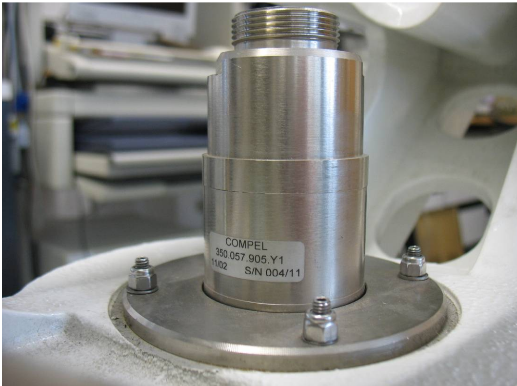
Photo No. 5: transceiver in-/output, antenna connector
