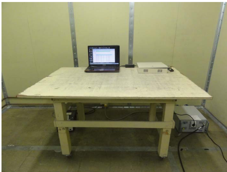
Photograph 3 : Setup for Conducted Emissions
