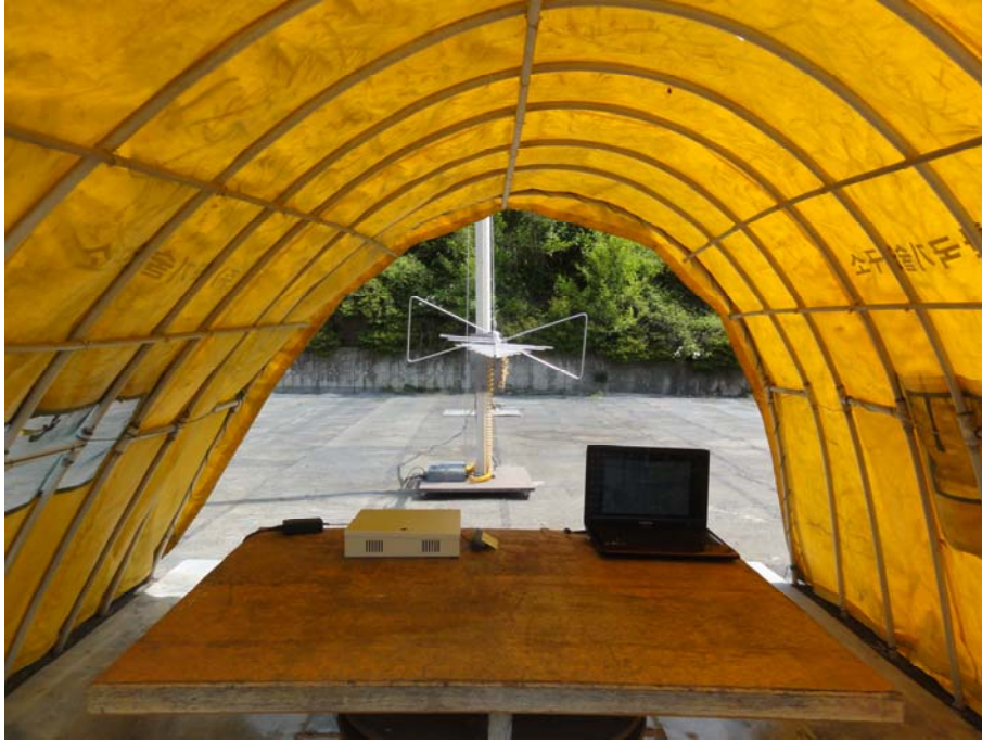
Photograph 2 : Setup for radiated Emissions (above 30 MHz)
