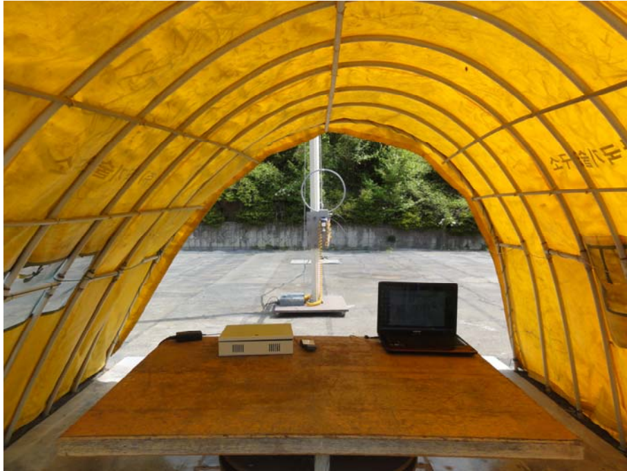
Photograph 1 : Setup for radiated Emissions (below 30 MHz)
