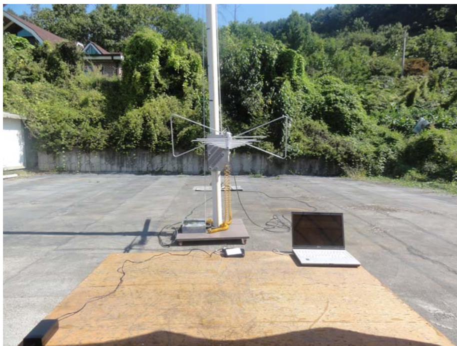
Photograph 2 : Setup for radiated Emissions (above 30 MHz)
