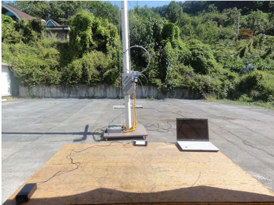
Photograph 1 : Setup for radiated Emissions (below 30 MHz)
