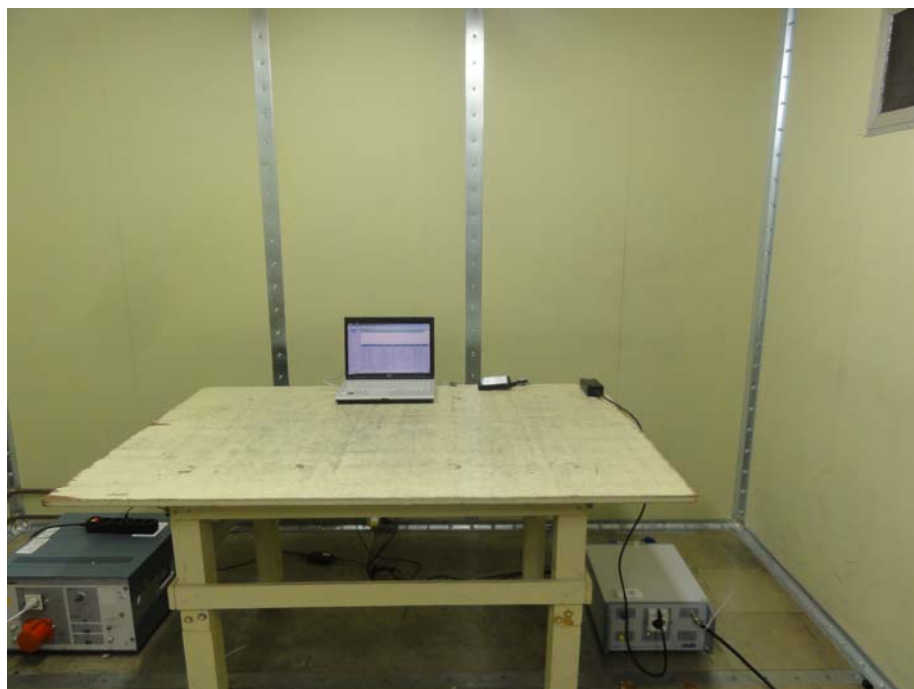
Photograph 3 : Setup for Conducted Emissions
