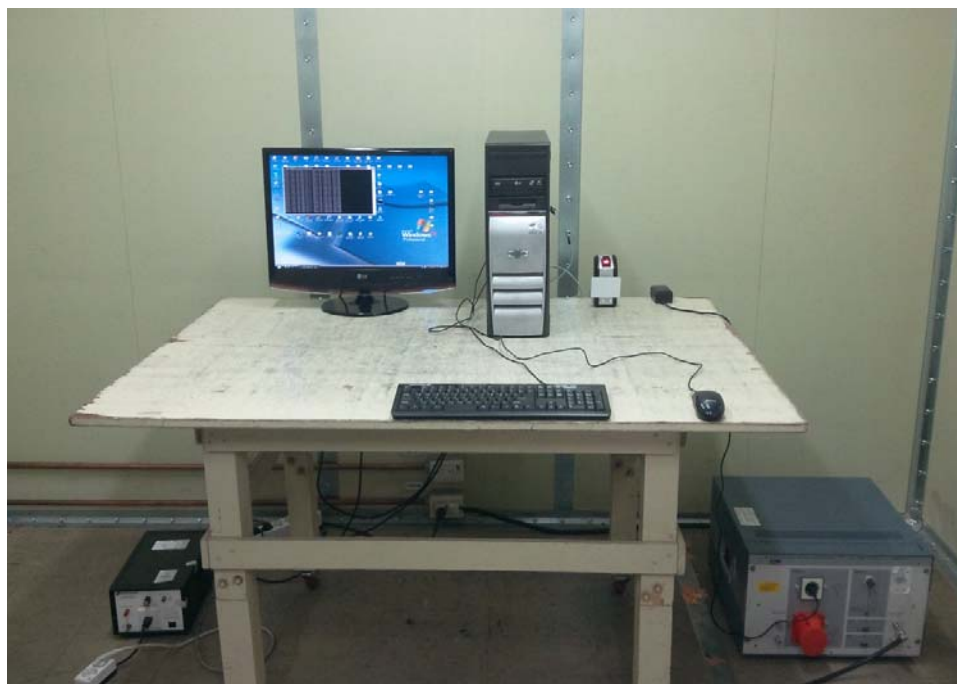
Photograph 3 : Setup for Conducted Emissions
