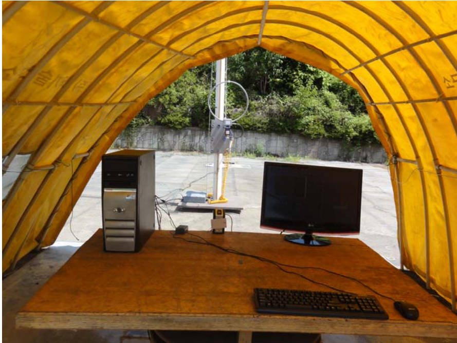
Photograph 1 : Setup for radiated Emissions (below 30 MHz)
