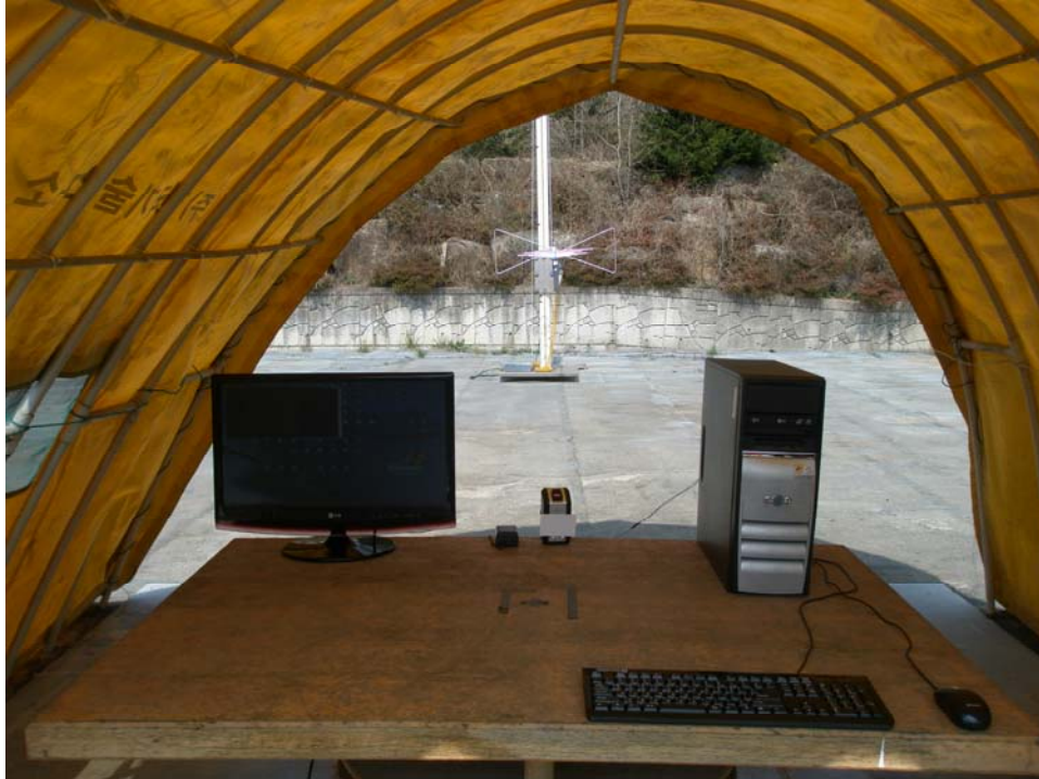
Photograph 2 : Setup for radiated Emissions (above 30 MHz)
