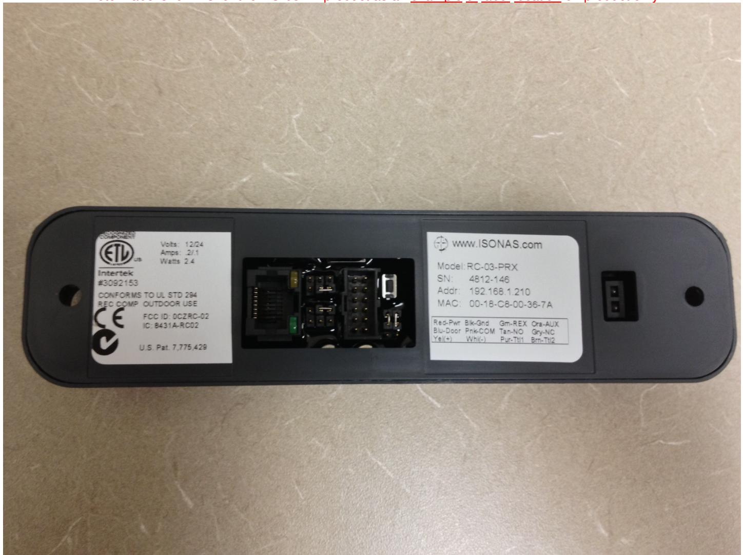
On the left side the distance from the existing label to the left edge of the controller is 0.6" which includes the mounting hole. On the right side the distance from the right side of the tamper window edge to the right side of the controller is 1" which also includes the mounting hole. The largest open spot is between the tamper window right edge to the mounting hole which is 0.5".
