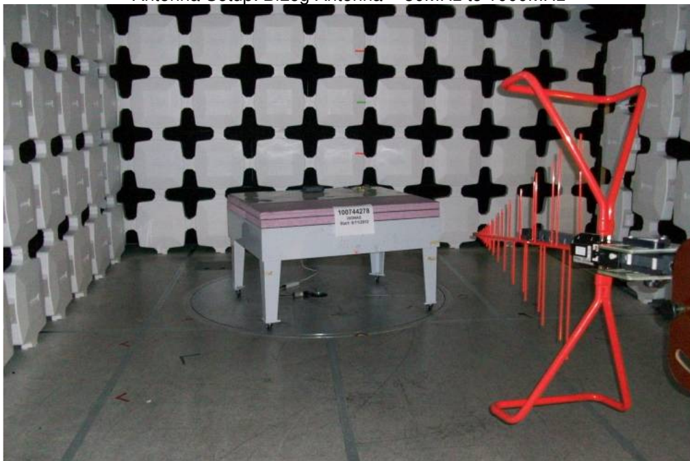
Antenna Setup: BiLog Antenna - 30MHz to 1000MHz
