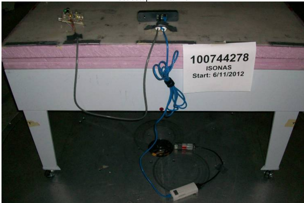
Midspan PSE located on floor
