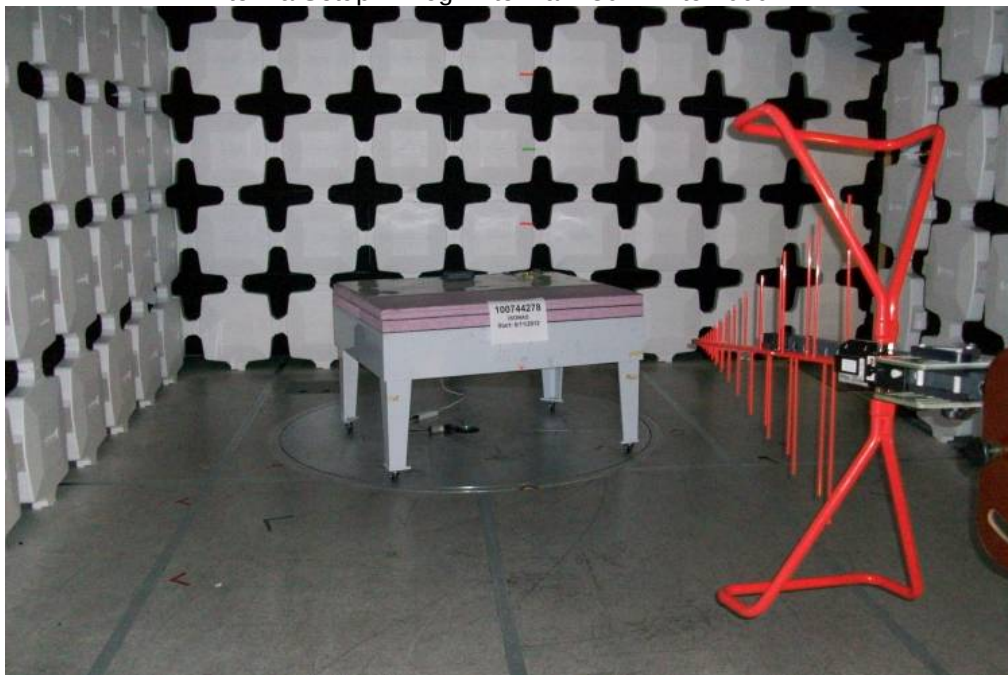
Antenna Setup: BiLog Antenna - 30MHz to 1000MHz
