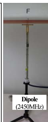
Test setup for the system performance check
