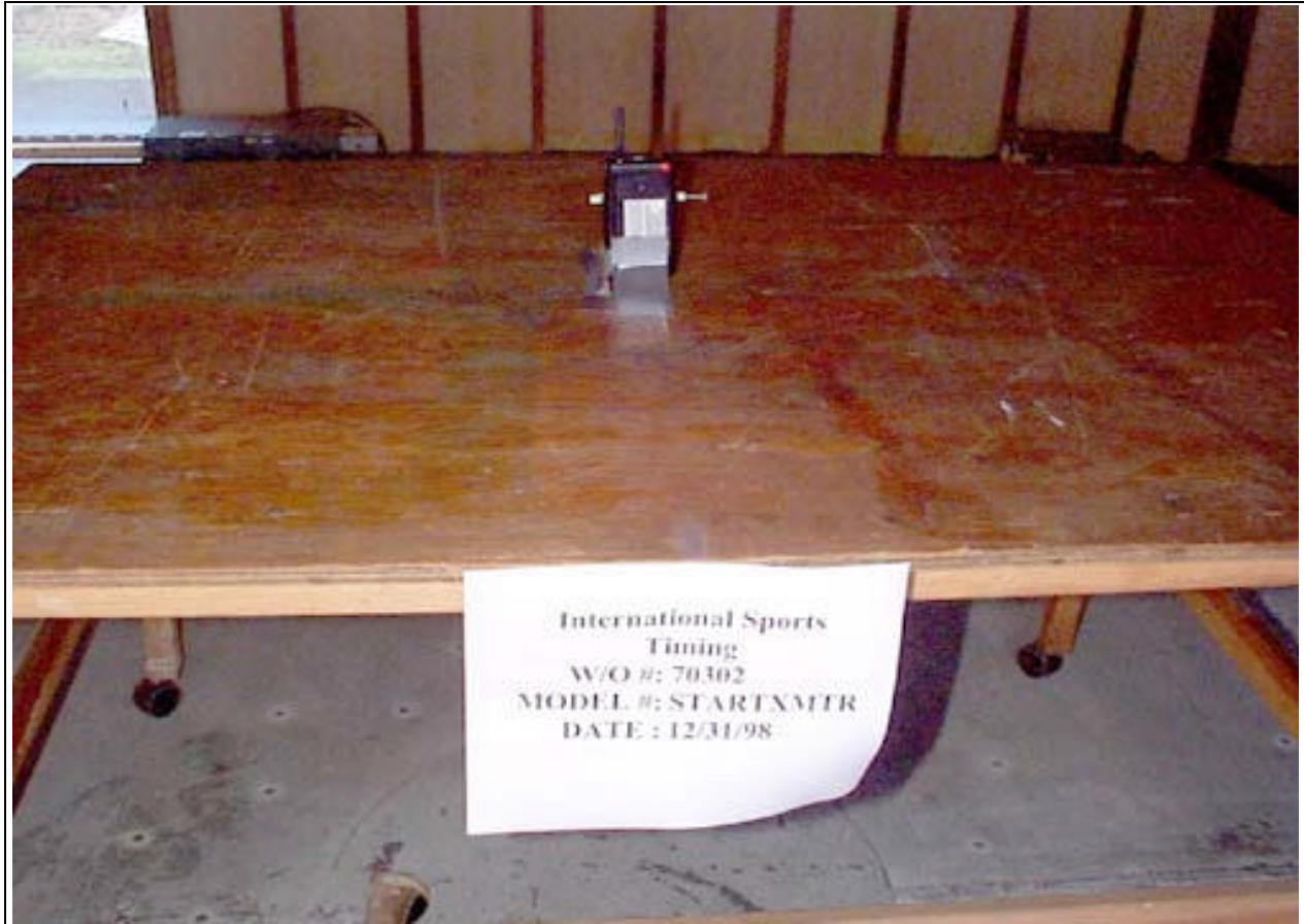
Radiated Emissions - Front View, Upright
