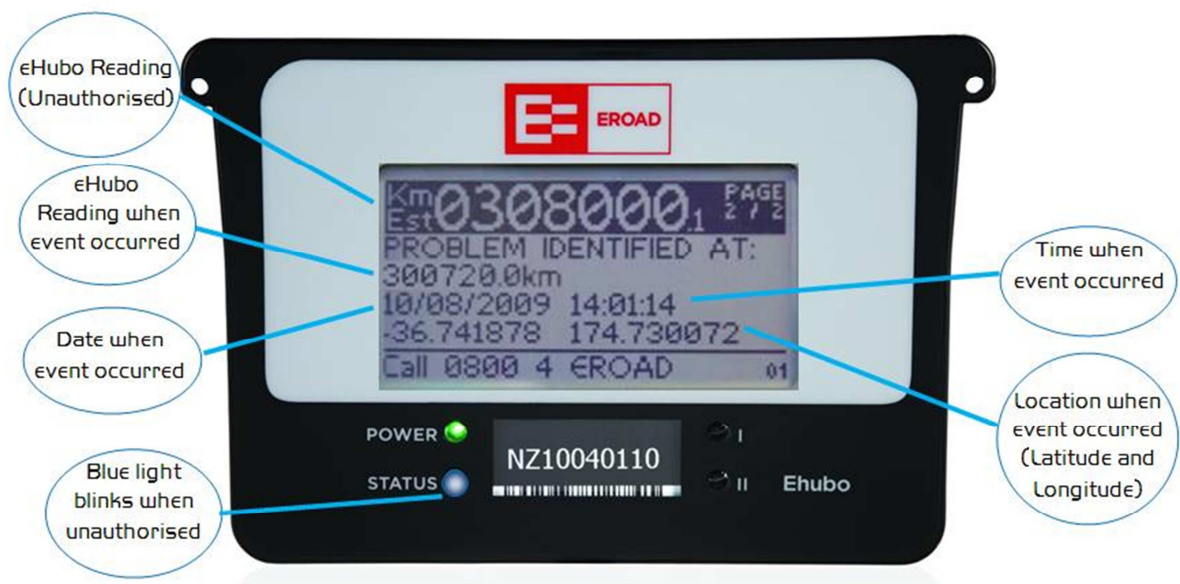
Figure 2 - Ehubo in Unauthorised Mode Displaying the Support Screen
