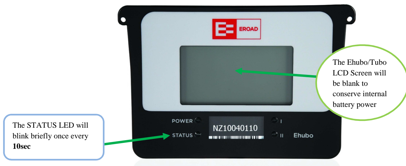
Figure 3 - Ehubo with External Power Disconnected
