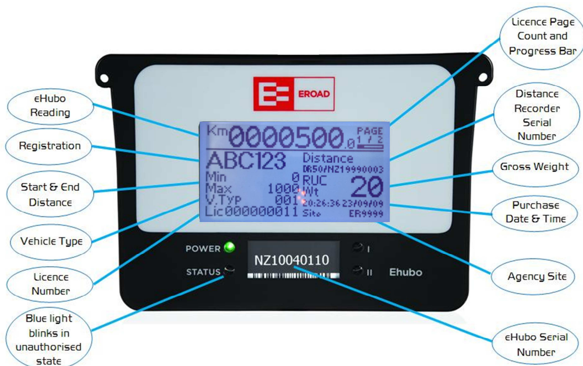
Figure 1 – Ehubo in Normal Operating Mode
