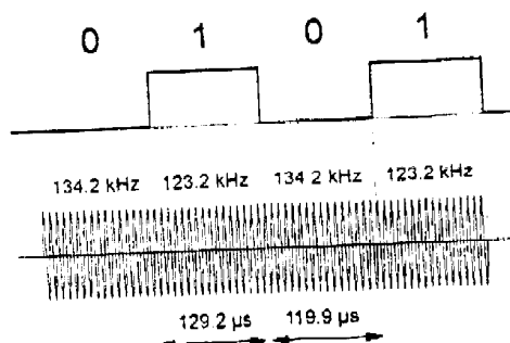
Figure 5: FM Principle Used for the Read Function of TIRIS Transponders
