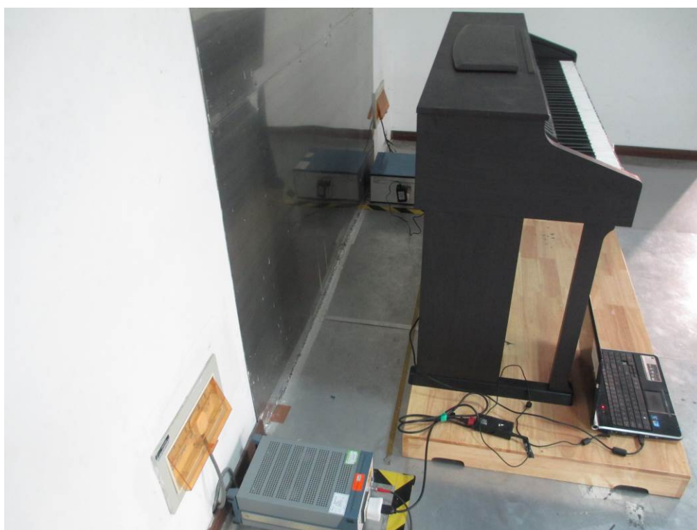
Conducted Emissions Test Setup Side View
