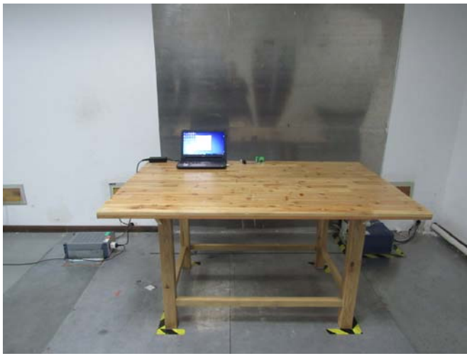
Conducted Emissions Test Setup Front View
