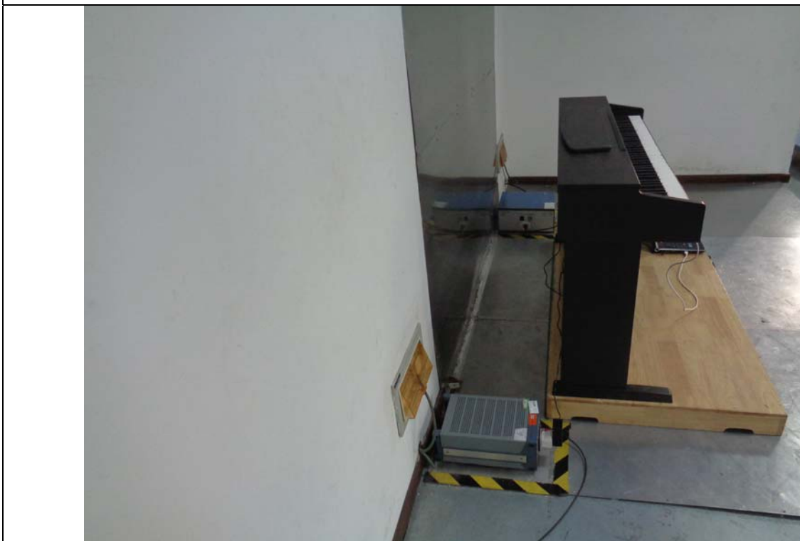
Conducted Emissions Setup Side View
