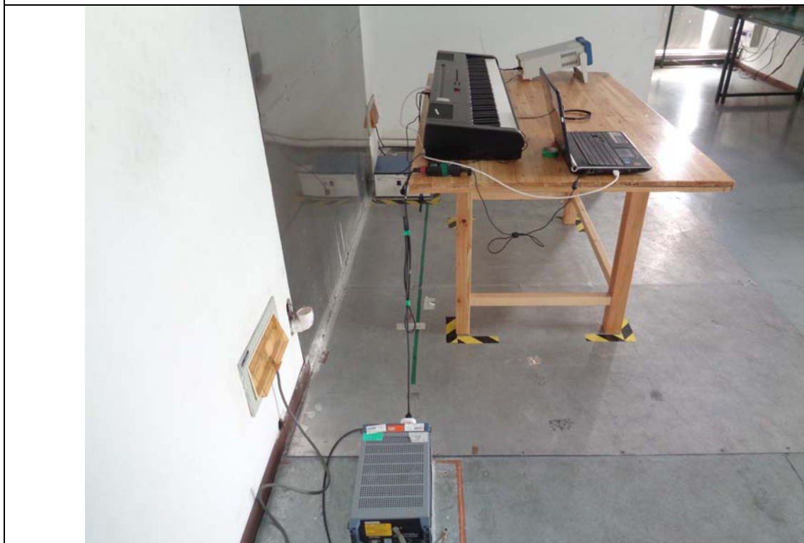
Conducted Emissions Setup Side View
